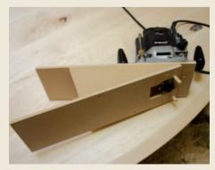
Surface Wealden's Surface Trim cutter has six wings with tungsten tips, and is ideal for skimming a wide bevel. The jig is simple to make from MDF, at about 23°, with the two dowels guiding it around a curved edge. Obviously you could make it adjustable if you wanted to use it for other jobs
