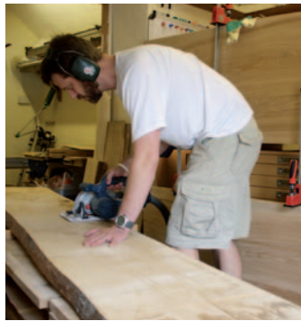
Pic.6 All the ripping was done on a bandsaw, which is better for following a 'chalked' line freehand than on a tablesaw. There is also less wastage in dust, and it's generally gentler. Steve is considering buying a rail-guided circular saw (like a Mafell or Festool) for dimensioning panels. The cordless Bosch saw wasn't quite strong enough for 2in ash boards, especially with a thin CMT blade, which is great for 18mm MDF, but wanders a bit in solid wood
