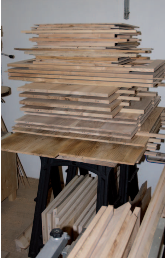
Pic.5 Stacks of panels back from the wide belt sander, in stick and hopefully staying flat. By doing all these at once Steve saves himself days of time, but the thicknesses have to be well planned to match cutters etc...
