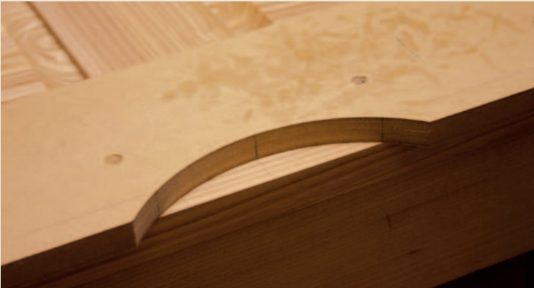
Jig Clamp a simple curved jig to the front face of the door to cut the recess. Steve used a guide bush on the bottom of his T11 router to shape the handles
