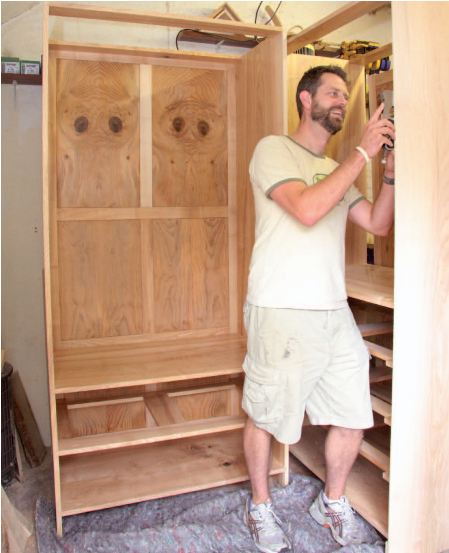
Fig. 1 Steve tidying up the rebate along the back edge of one wardrobe with a shoulder plane to fit the back panel
