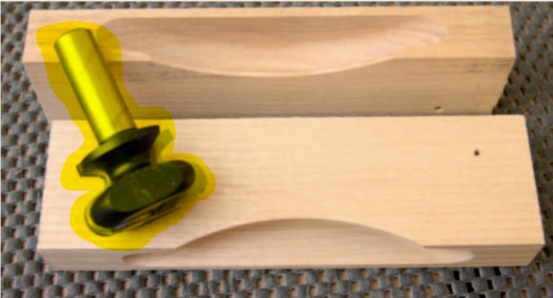
Jig Clamp a simple curved jig to the front face of the door to cut the recess. Steve used a guide bush on the bottom of his T11 router to shape the handles
