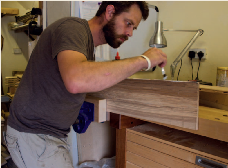
Pic.8 Applying Evo-Stick PVA with a brush to one of the door panels
