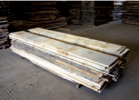
Pic.2 Vastern's had prepared Steve a pile of boards (above) for him to sort through at his leisure. This is a great luxury for any woodworker. In particular he was looking for flat boards (right) for the 8in-wide pieces that he needed to glue up the carcass sides (C). Gradually he moved the boards he wanted from Vastern's stack onto bearers of his own to keep them safe from bruising on the concrete floor. Ultimately he had to return because he forgot the 11/2in boards for the drawer fronts, but fortunately Vastern's are close to our workshops
