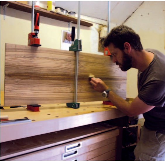
Pic.4 Cleaning up the book-matched boards for one of the ash door panels. The door panels are 15mm thick, with fielding on the front and a shaped rebate on the back. Steve used a panel raising cutter for the front and a drawer pull cutter for the back, to size the tongue accurately to fit in a 6mm groove in the door stiles (N) and rails (O). Wealden produce a combined Back Cutter Kit (T1960, wealdentool.com) to go with their panel raising cutters to produce a guaranteed 6mm tongue even if the thickness of your panel is inconsistent because you always work off the front face of the panel, with that face down on the router table. The cedar panels (M) in the back are 12mm thick. They are flat on the inside, but rebated on the rear to fit in the 6mm groove in the back rails & stiles
