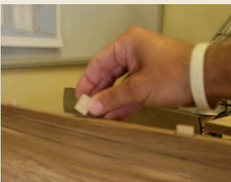
Pic.7 Using Dominos to locate the edges on the panels. This means there's less waste to be removed later
