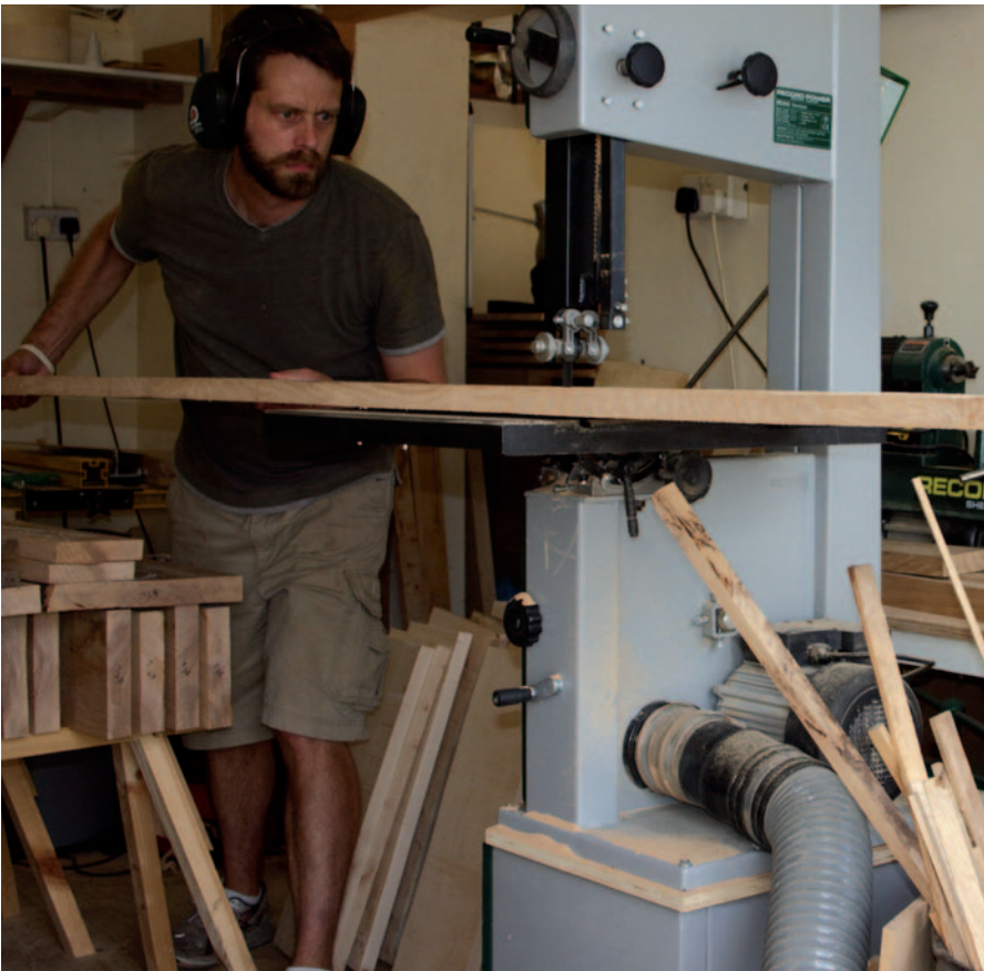
Pic.4 Cleaning up the book-matched boards for one of the ash door panels. The door panels are 15mm thick, with fielding on the front and a shaped rebate on the back. Steve used a panel raising cutter for the front and a drawer pull cutter for the back, to size the tongue accurately to fit in a 6mm groove in the door stiles (N) and rails (O). Wealden produce a combined Back Cutter Kit (T1960, wealdentool.com) to go with their panel raising cutters to produce a guaranteed 6mm tongue even if the thickness of your panel is inconsistent because you always work off the front face of the panel, with that face down on the router table. The cedar panels (M) in the back are 12mm thick. They are flat on the inside, but rebated on the rear to fit in the 6mm groove in the back rails & stiles
