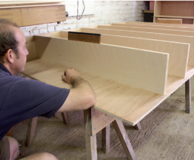
Pic.1 The 15mm-thick ply back stabilises the bookcases because at 18mm the shelves are relatively thin and could flex without good support. They are glued and screwed to the back with long 50mm screws to stop bowing (above right)
