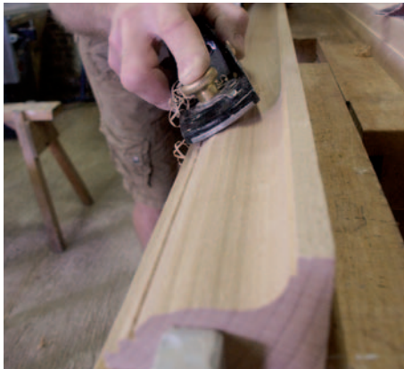
Pic.6 To create this short length of cornice, Gordon used a series of cutters. First he uses straight ones to form the three steps (or quirks). Then he removes as much of the waste as possible with straight cutters from the concave section until he has to use radius cutters to follow the curve. Then he planes away the convex section. It's a bit trial and error, but cheaper than getting cutters made
