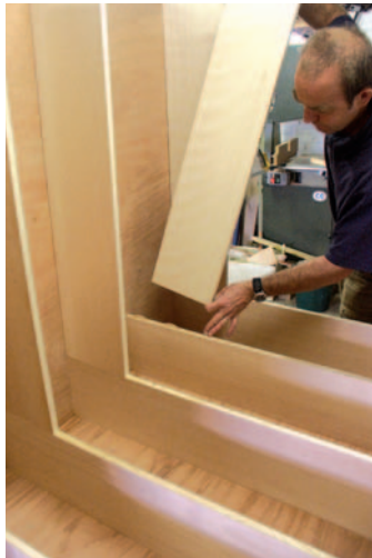
Pic.2 The L-shaped section is delivered on site in two parts. In the workshop Gordon glues and screws the shelves to the backs, and in each case biscuit joints one end panel to the ends of the shelves. The back panel is glued and screwed into a rebate down the back edge. The rebate (left) is extra long so that it can be scribed into the wobbly wall. With one lot of shelves screwed to a back, and an end panel fixed, you can present the second unit up to position the shelves. The ends of these shelves (vertical on the right) are biscuit into the front edge of the horizontal shelves, and will be glued in place on site
