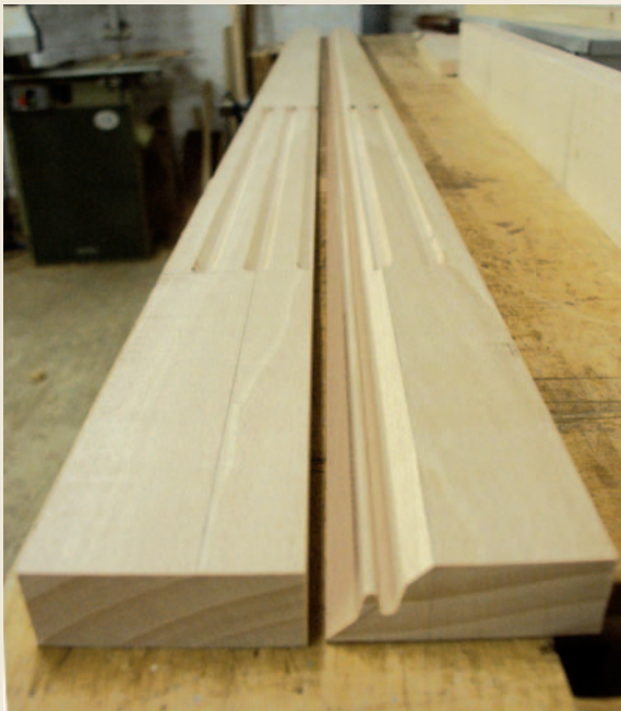
Pic.9 Aligning the mitre lock joint with the flutes. The first half of the mitre has been cut down the centre of one flute. Gordon has marked out where the second mitre cut will go, straight down a flute on the other piece. Once the L-shaped cover strip has been assembled (below) only three flutes will be visible, to match the three flutes on the end cover strips (Pic.6)
