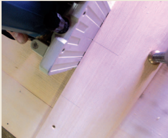
Pic.5 The jointer set square also gives you an 18mm stop against which to rest the biscuit jointer for more stable working (above left). Gordon does a lot of his assembly and large work on his tablesaw top (above right). He has a swing arm crown guard, which cost £300-400, but has saved him huge amounts of time in his smallish workshop. He thinks it used to take him 20 minutes to remove the crown guard and riving knife to lower the blade so that he could use the tabletop for other uses. Now it takes him seconds. The riving knife is never removed, but stays just a fraction below the height of the top teeth
