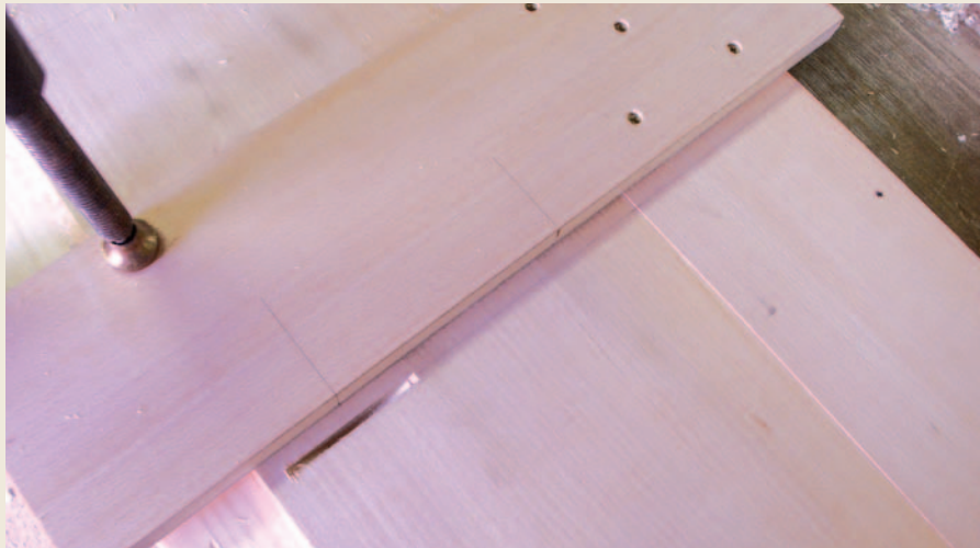
Pic.4 The jointer set square is screwed and glued. Apply glue and insert one screw first, then check for square and insert the other screws. That way the shelves will be flat
