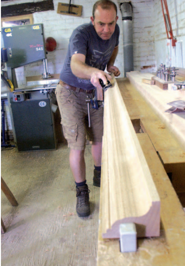
Pic.6 To create this short length of cornice, Gordon used a series of cutters. First he uses straight ones to form the three steps (or quirks). Then he removes as much of the waste as possible with straight cutters from the concave section until he has to use radius cutters to follow the curve. Then he planes away the convex section. It's a bit trial and error, but cheaper than getting cutters made
