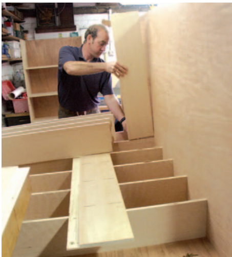
Pic.3 Presenting the second set of shelves to form the L-shape in the workshop. The vertical back is screwed to the end of the horizontal shelves during this dry assembly
