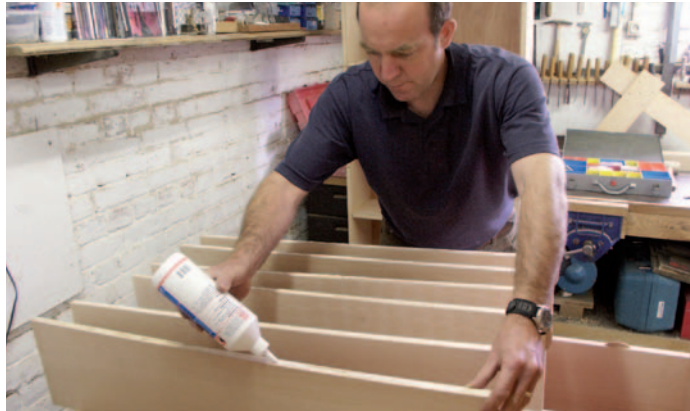
Pic.1 The 15mm-thick ply back stabilises the bookcases because at 18mm the shelves are relatively thin and could flex without good support. They are glued and screwed to the back with long 50mm screws to stop bowing (above right)
