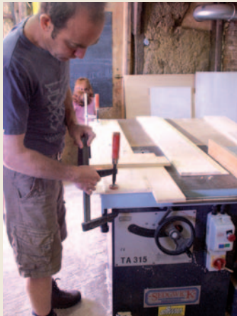
Pic.5 The jointer set square also gives you an 18mm stop against which to rest the biscuit jointer for more stable working (above left). Gordon does a lot of his assembly and large work on his tablesaw top (above right). He has a swing arm crown guard, which cost £300-400, but has saved him huge amounts of time in his smallish workshop. He thinks it used to take him 20 minutes to remove the crown guard and riving knife to lower the blade so that he could use the tabletop for other uses. Now it takes him seconds. The riving knife is never removed, but stays just a fraction below the height of the top teeth
