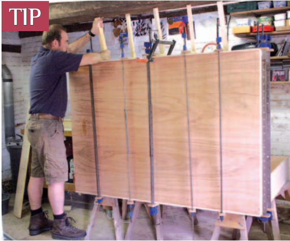
Pic.7 Unlike on site where you often can't use cramps, at least in the workshop you have access to all your tools. Even then, you have to improvise sometimes. With the L-shaped bookcase dry assembled (left) Gordon has to fix the end panel onto the vertical set of shelves. He can put long sash cramps at the back (facing us), but cannot do so for the internal edge of the end panel. So he uses Go Bars. These are lengths of wood, just a bit too long, which are wedged between the beam and the top face of the end panel
