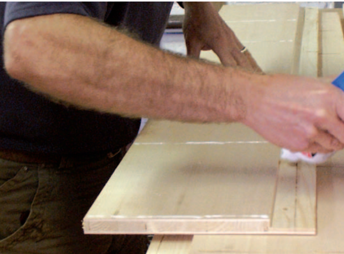
Pic.2 The L-shaped section is delivered on site in two parts. In the workshop Gordon glues and screws the shelves to the backs, and in each case biscuit joints one end panel to the ends of the shelves. The back panel is glued and screwed into a rebate down the back edge. The rebate (left) is extra long so that it can be scribed into the wobbly wall. With one lot of shelves screwed to a back, and an end panel fixed, you can present the second unit up to position the shelves. The ends of these shelves (vertical on the right) are biscuit into the front edge of the horizontal shelves, and will be glued in place on site
