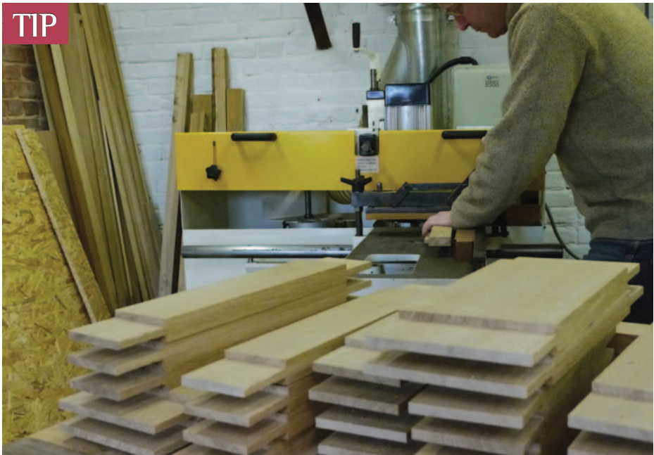
Pic.4 As the tenons on the rails were to be all the same length, the stop point on the Sedgwick tenoner was set for the entire project, which enabled me to pass all of the rails at the same time (above). There are four tenons to each shutter, making a total of 80 tenons in all which took less than an hour all told. It takes about 10 minutes to set up the tenoner, but 30 minutes if I am using a scribing head as well. I always machine spare spock for the setting-up process. Marking the haunch point on the tenon (right)
