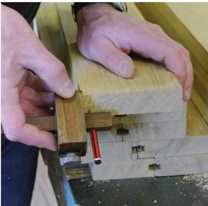
Pic.1 Using a marking gauge to mark the haunches on the stiles (above). The mortise chisel is wider than the 7mm groove, so I marked it to cut a sharp joint. The cut-depth for the mortise was 65mm, so a 7/16in (11.11mm) chisel extending to 70mm does the job (right)
