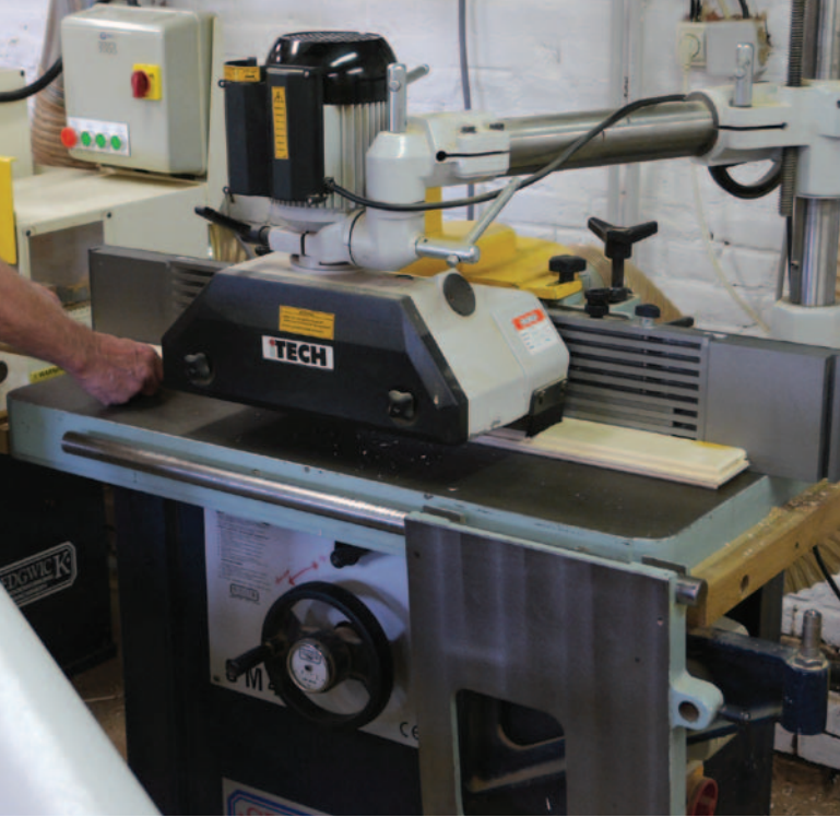
Pic.4 I used the Trend RT/80 on a 1/2in shank (£58.76+ VAT from Wealden) in order to cut the 45° on the end-grain of the panels (above). This cutter has four edges to work and due to the disposable blade system, the same profile can be achieved each time. I bought mine in 2008, and, although I have changed the blade in that time, this cutter has held up incredibly well. I also purchased the bearing and collar at the same time and have used that on templating jobs. Some of the pre-made T&G boards had to be cut down to give continuity to the design across the width, so after cutting a 45° chamfer on the end-grain, they were then passed through the Sedgwick spindle moulder to re-cut the 45° chamfer on the long-grain and to re-cut the groove (right)
