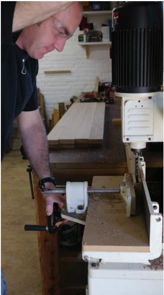
Pic.1 Using a marking gauge to mark the haunches on the stiles (above). The mortise chisel is wider than the 7mm groove, so I marked it to cut a sharp joint. The cut-depth for the mortise was 65mm, so a 7/16in (11.11mm) chisel extending to 70mm does the job (right)
