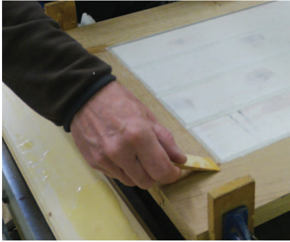
Pic.7 You don't have to hit very hard with a hammer like this (above)! It is a flooring mallet, which I bought several years ago with a power floor nailer. Adjusting the spacing to 3mm between boards to allow for swelling and shrinkage (left)
