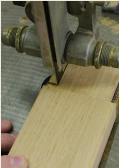
Pic.6 Testing the fit of of the T&G board. I use Rustins Knotting (rustins.eu). I always use it on softwood, where sap is the main enemy. All the shutters are to be painted, so I made sure to prime the tongues and grooves before assembly. I did not paint the tenons on the oak frames as these were to be glued
