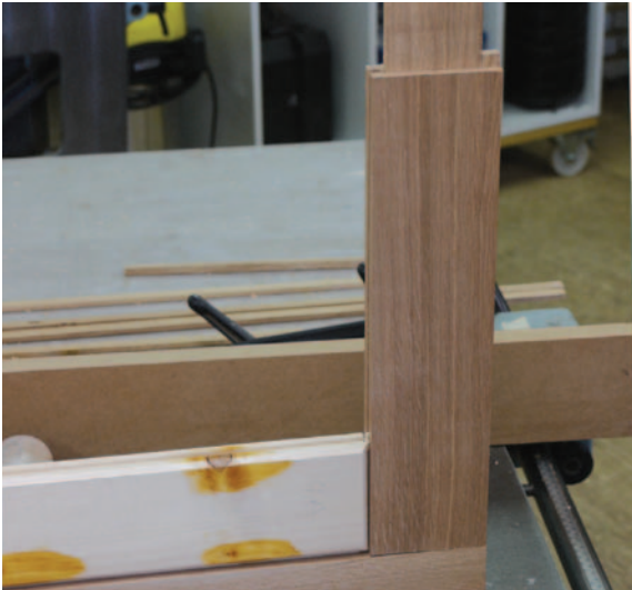
Pic.6 Testing the fit of of the T&G board. I use Rustins Knotting (rustins.eu). I always use it on softwood, where sap is the main enemy. All the shutters are to be painted, so I made sure to prime the tongues and grooves before assembly. I did not paint the tenons on the oak frames as these were to be glued
