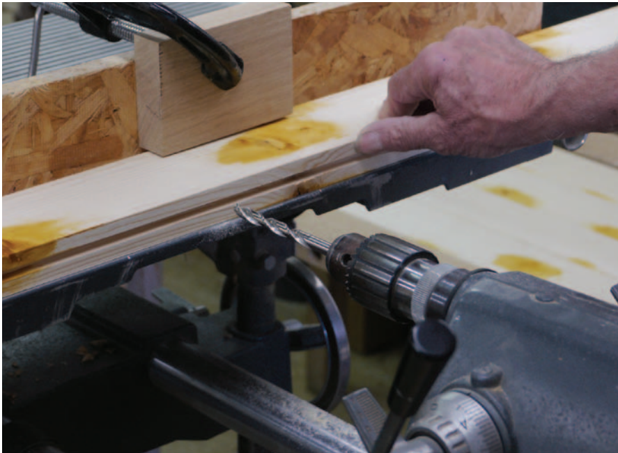
Pic.4 I used the Trend RT/80 on a 1/2in shank (£58.76+ VAT from Wealden) in order to cut the 45° on the end-grain of the panels (above). This cutter has four edges to work and due to the disposable blade system, the same profile can be achieved each time. I bought mine in 2008, and, although I have changed the blade in that time, this cutter has held up incredibly well. I also purchased the bearing and collar at the same time and have used that on templating jobs. Some of the pre-made T&G boards had to be cut down to give continuity to the design across the width, so after cutting a 45° chamfer on the end-grain, they were then passed through the Sedgwick spindle moulder to re-cut the 45° chamfer on the long-grain and to re-cut the groove (right)
