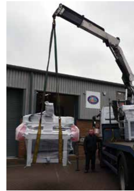
Offloading new CNC machine using Hiab
