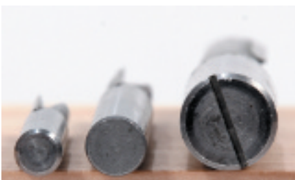
3. Cutters with 1/4in, 8mm, and 1/2in diameter shanks
