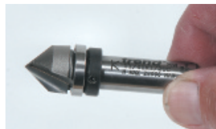
4. The 'K' mark on a cutter shank indicates how far the shank should be inserted in the collet
