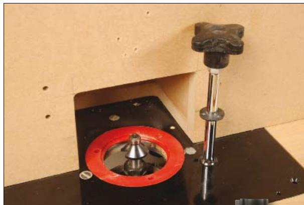
The Trend T11 comes with a winding handle for easy and accurate height adjustment in a router table
