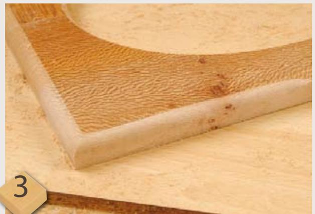
Repeated the process on the outer edge, this time with the cutter height set to give a roundover which can be sanded smooth afterwards
