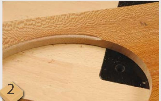
A part moulded inner profile with the cutter set down to create a step. On the front you can use two moulding treatments: one to bevel or roundover the inside of the ellipse cutout; the other to mould the outer frame edge if you want to do that too
