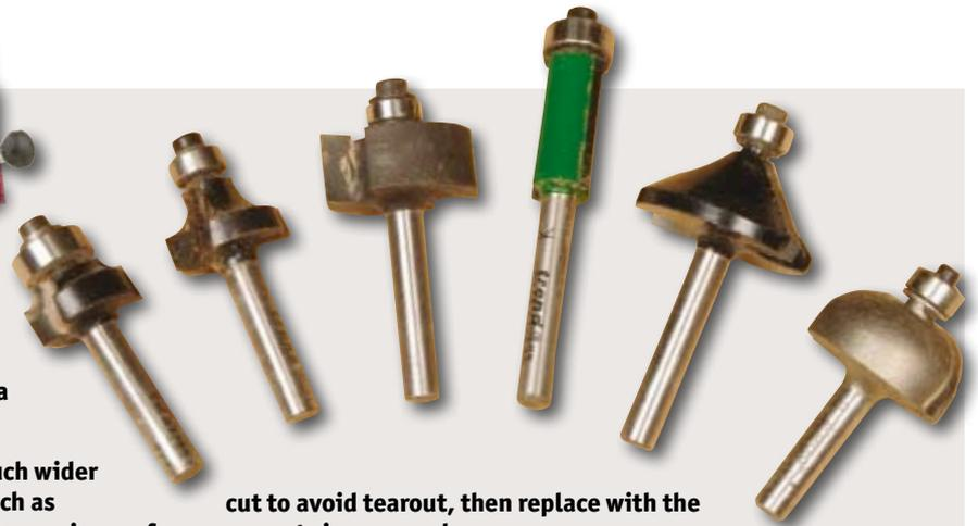
The cutters shown will create this frame design. From left to right there are two sizes of **roundover**, a small **rebater**, a bottom mounted bearing guided trimmer, a **bevel** and a cove cutter.
