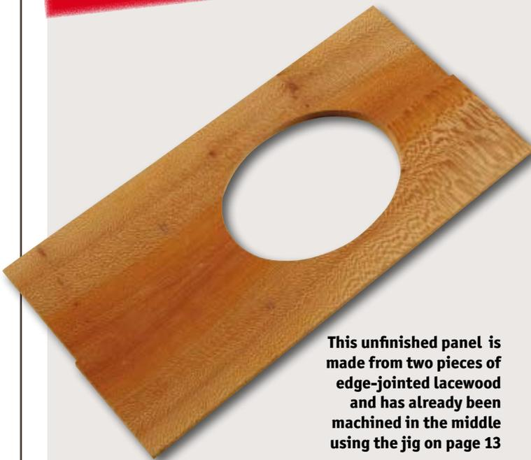
This unfinished panel is made from two pieces of edge-jointed lacewood and has already been machined in the middle using the jig on page 13
