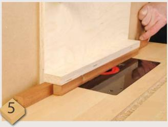
You need to experiment to get the tunnel positioned correctly over the cutter, so do some test cuts until it is right. You will find vibration drops considerably, improving the cut finish and preventing the workpiece jumping and causing damage. It will therefore lessen the shock caused to small straight cutters that might otherwise break, and avoids any risk to your fingers
