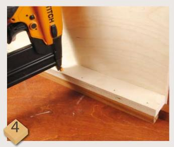
Now with the component and the length of component offcut pressed firmly in place, pin that offcut to the strip of ply. You should now have an inverted 'U' shaped tunnel which will enclose the components you are about to machine
