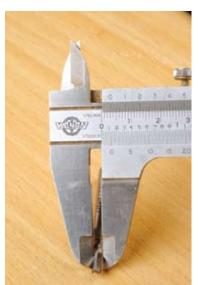
Measuring the cutter diameter
