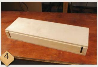
Cut two pieces of 9mm or 12mm birch ply to fit inside the base pieces and four offcuts of softwood all glued together to create a box around which the facings will be glued. The top piece of ply is narrower to create a rebate for the cabinet back panel. The softwood and plies must be flush all round apart from this – check with a square after clamping up
