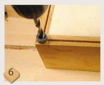
All the location dowel holes are drilled in the top and base. Use a dowel pin to mark the ends of the glazing bars and drill those holes. The back panel is now glued and pinned into the base rebate and checked for square. The rear glazing bars can also be dowelled in place and glued to the back panel
