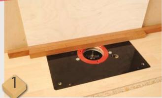
Clamp a sheet of ply or MDF in across the cutter, opening on the router table to create the through fence. Machine all the components to the same size using a thicknesser for accuracy. Lay one piece against the through fence and a second shorter piece next to it
