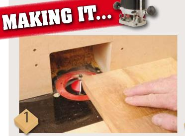
Decide what size the cabinet needs to be – this is governed by internal height, width and depth sufficient to contain the trophies. Cut the cabinet top to size including the extra amount for the projecting edges. Set up a large bevel cutter in the router table and do the bevel edge in several passes to depth. In this case, you can alter both cut depth and width as you work towards the final cut
