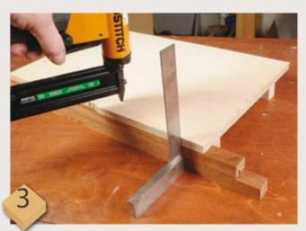
Remove the ply through fence and pin the narrow piece of ply to it using another piece for support while you do so. Use a try square and the intended component and the offcut to get the positioning correct. Note that the tunnel must fit tightly around the pieces you are going to machine
