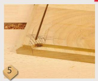
The top has a rebate machined at the back to accept the birch ply back panel, as do the two rear glazing bars
