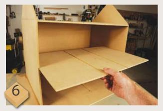
Butt glue the outer walls together, and onto the baseboard as well. Dolls' houses are generally done without more complex joints because of the relative simplicity. Slide the floor, ceiling and walls into place with some glue brushed onto the edges first
