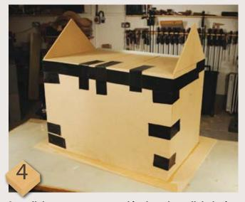
Once all the components are machined, you have all the basic outer parts you will need. Do a trial dry assembly using duct tape, so you can make sure everything fit together properly
