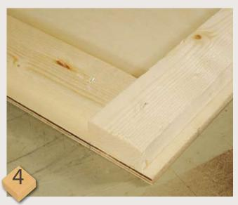
Fit a fillet of wood on each edge underneath the template so the board you are going to machine is trapped in the middle
