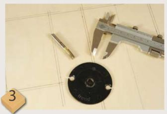
You need to calculate the difference between the cutter and guidebush diameters, divide it and add this amount to the size of all window and door openings
