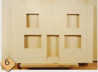
The finished template can be used over and over again, and machining the dolls' house front will take just minutes to do, so you make as many as you like very quickly
