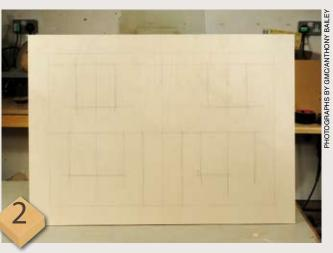
Mark out each template with window and door openings. You can have more openings than you finally use – simply ignore the ones you don't want but machine out the others
