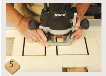
Rout out each opening in one or two passes depending on how comfortable the router feels – don't strain the cutter or motor. Use a straightedge or a clamp-on guide for accurate slots. Sit the board being machined on battens so that the cutter can go right through easily
