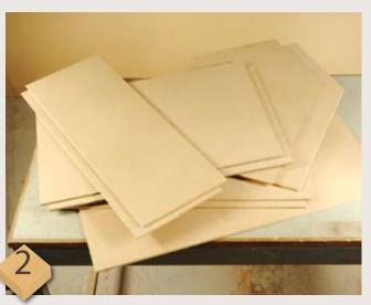
The baseboard is square, as are the roof panels. The back may also be a plain square, so all these can be cut very neatly with a saw, as can the gable ends of the building. Note that square meeting edges are important because these will slmply be butt glued with PVA
