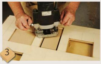
Use each template with a small guidebush and a 6.4mm straight cutter so you get the squarest corners possible. Use an extractor to clear dust away and allow the guidebush to move tightly into the template corners without dust packing them out and spoiling the line of the cut
