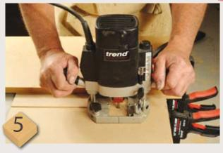
Mark the floor and ceiling positions on the inside of the walls, and use a straight cutter and a router T-square to make shallow grooves for the floor and ceiling to slide into. Cut and fit the floor and repeat the grooving operation for the inner walls, ensuring you copy the marks across between components so the grooves will line up correctly. The walls will need door openings and the floors stair access, of course
