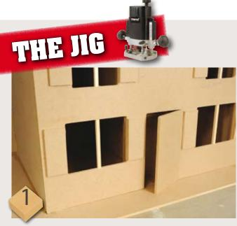
The jig is most important for making the front of the dolls' house. We have door and window openings that the router can easily machine. Likewise, you could have a rooflight (window) in one of the roof panels, again routed
