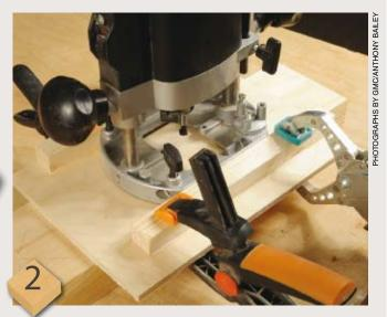
Glue and fix battens in place onto your plywood base so they allow the router to move in one direction only
