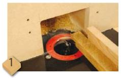
marring the finish. Where a cutter will be partly behind the fence line, fit a sub-fence and start with the cutter well behind it. Switch on and push the fence back carefully until the cutter breaks through and is exposed enough for the cut you need. Keep hold of the fence and press the NVR switch to cut the power. It is best to keep hold of the fence for this, so have a friend switch it off for you. This is because snatches
