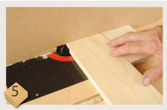
Use a tenoning cutter, or a 19mm straight cutter with a through fence in place to machine a rebate on the ends of the cabinet side pieces. Use a square cut push block behind for accurate support and to avoid breakout
