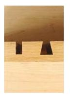
To remove the bulk of the waste, first use a straight cutter that is narrower than the width of the opening into the joint, and do repeated passes to near final depth. Fit the desired necked cutter and make the cut from the end, thus creating the final profile while taking out a minimal amount of wood. It avoids burning, chip clogging, and cutter breakage, plus it improves blade life and your working experience.
