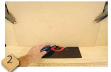
and kickback occur at slower speeds, and you need the fence to stay put. If there is a bearing or shaft on top of the cutter you need to cut this area out with a bandsaw first. Your subfence is now ready and you can wind the cutter up or down while running. Trim away any fluffing or tearout at the outfeed side of the cutter with the router switched off. Email your router questions to:
