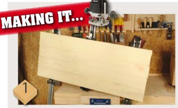
Cut and plane all components to width and length, except for top and bottom pieces and the door, which is trimmed to size later. If using solid wood for this you may need to carefully edge joint pieces together for the door and back panel – which should be thick enough to accommodate the piano hooks
