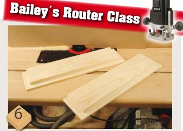
The cabinet sides are also rebated so they sit along the sides of the back panel without projecting too far, for aesthetic purposes. Do this at the same cutter and fence settings
