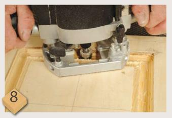
The door is cut to size and a template made for the bearing guided face moulding cutter (see Router Class in WPP43 for more on template working). Make sure you use an offcut in the middle for support and keep the router tight to the edge of the template and machine at an even pace. The template is pinned to the door blank and the blank sits on a rubber router mat. The edge has an ovolo shape routed on it. Finally sand, apply a finish, and fit the hooks, hinges, knob and a catch!
