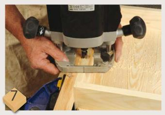
Now cut the top and bottom to fit when the side pieces are in place. All components can be sanded and glued and pinned in place. For simplicity, the hinge recesses can be machined to the full depth of the folded hinge into the cabinet carcass, and simply surface fixed to the door. You don't need a jig for just two recesses, but you do need to clamp a batten along the cabinet side to give more support for the router and fence
