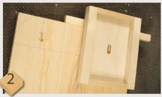
Mark out the cabinet top position on the backboard and the shape for the projecting top, also the keyhole positions on the reverse side. Use the keyhole jig to machine the keyhole slots while the top is still square
