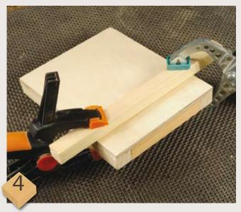
Place the tray jig on the back panel to ascertain the correct position and then fit a crosswise batten underneath the tray jig at the chosen position
