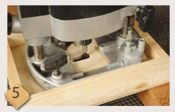
With the jig resting on battens lifting it clear off the bench, place the router at the top end of the tray jig. Switch on and plunge the cutter so the widest part that will create the keyhole entry point goes into the jig base, and slide the router along to create the full length slot – you may need a deeper second pass to machine right through. You now have visual access of the slotting area and the jig is ready for use on the back panel of the cabinet
