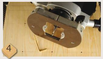
To make accurate holes for the piano hooks that hold the keys, a 3mm spiral cutter is ideal for drilling with the router. Use some abrasive taped to the baseplate if necessary, to stop the router from wandering
