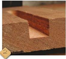
If one face is more critical than another, i.e. a 'seen face', then unlock one fence rod and tap the unplunged router over fractionally, lock and re-pass at full depth for a fulldepth clean finish.
