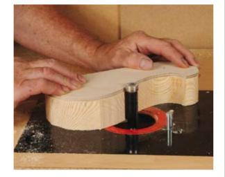
Many different tasks can be done depending on the size of router and cutter in use, even 50mm-thick electric guitar bodies, or other big sections such as brackets, can be made this way
