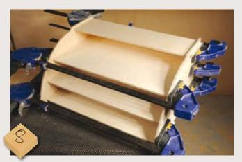
Dry assemble the rack and measure and cut out both the base and dividers to suit. Notch out the top corners of the dividers so the ends fit in the housings. Sand and assemble the magazine rack with PVA glue, when dry apply a suitable finish and the job is done
