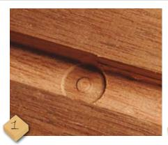
router gently as you start the cut. As regards 'offline stepping', this is often worse when using a trammel to cut circles but can happen with straight cuts as well. Make sure your whole setup is locked tightly for a start, e.g. fence rods and plunge lock, as routers can waggle on the columns when unlocked.
