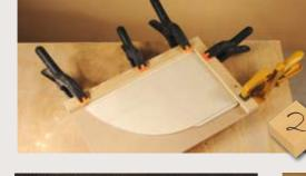
The jig is made from 6mm MDF and softwood battens, which are clamped then screwed in place along two sides with a prepared rack side in place. The battens are clamped first before the jig is turned over for insertion of the screws
