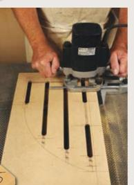
A 16mm straight cutter was used to create slots for a 16mm guide bush using a straight fence and taking care not to let the cutter deviate off course
