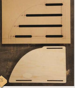
Use the end jig to make the long slots in each end component so the ply tenons can slide into them using a 16mm guide bush and 6.4mm straight cutter combination
