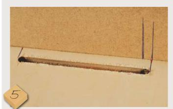
Next, cut out the front and back allowing for the projecting tenons. Mark out the tenons and make the long cuts between on the router table doing a 'drop-on' cut with the 6.4mm straight cutter, starting where each slot begins, and lift off once you reach the end of the slot. Put marks on the through fence so you can see where the cutter is. Do the short shoulder cuts with a fine-tooth handsaw and round the ends with a chisel so they fit in the mortises
