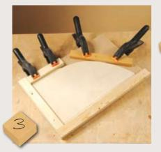
Fit two other battens in place so the end blank is held firmly. Now remove the blank ready for marking out
