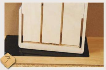
The resulting bottom panel groove neatly meets up with the other slots and grooves
