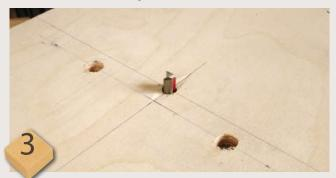
Assemble the table with blocks underneath the top joints to reinforce it, as only butt glue joints are used. Once dry, mark and drill to accept the fixing holes on your router. Mount your router, minus fine adjuster, with the straight cutter you will use for the finger joints, and plunge-cut through the surface. Unplunge and switch off
