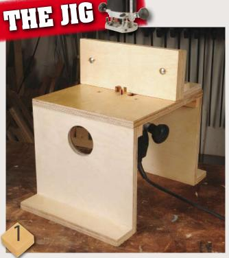
The caddy box uses finger joints for their looks, while being strong enough to hold the box together. Finger jointing requires a special jig that once built, is easy to use and can be used time and again. The jig resembles a small router table
