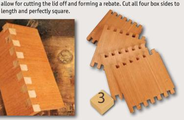
Mark the joint pairs so you ensure the halves all match together correctly. And once you have cut all the joints, do a dry assembly to confirm all the pieces fit together nicely
