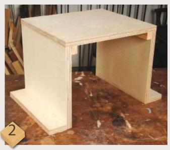
Cut out the pieces to make the inverted U-shaped table. The dimensions are not exact but you need to take into account the unplunged height of your router with a fine adjuster fitted. The table needs to be wide enough to support workpieces and long enough for the sliding fence to move forward each time you cut a slot
