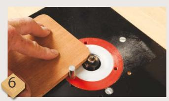
Round the corners of the top and bottom components so they will sit neatly in the box rebates. Rebate them, this time using a lead-in pin to start the cut. Take care to check the top and bottom will fit tightly into the box sides and flush when fully inserted. Glue the top and bottom in place
