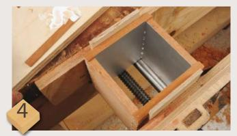
Before gluing the box up, use spray mount adhesive to stick kitchen foil, matt side out, on all the inner caddy box faces. Trim it off the actual fingerjoints. Glue and clamp the box together using pads narrow enough to sit inside where the fingers are so the box will close up properly. Repeat on both sides, check for square and remove glue with a soft damp cloth. You then need to level the sides, front and back
