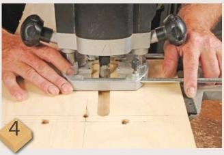
Demount the router and use a 19mm straight cutter and straight fence to make an accurate slot to the side of the cutter hole in the table. This slot will accept the batten on which the fence is guided, so it needs to be a good fit
