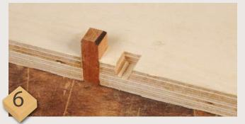
The last and rather vital component is a peg that is the same width as the cutter, and a height just slightly less than the finger height of the joints. This is mounted in the sub fence at the fingerjoint width to the side of the recess to take the router cutter. When making both the cutter slot and peg slot, hold a thin piece of ply tight to the sub fence to avoid any breakout. Finish the peg slot with a fine handsaw and glue the peg in place
