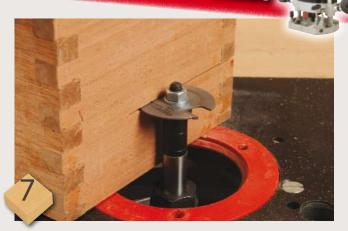
Decide where to separate the lid section, preferably on the join between fingers. Do this with a 1.5mm groover so removing a minimal amount of wood. A bearing should be fitted that has a diameter sufficient to prevent complete separation – this avoids the box dropping onto the cutter and spoiling the job. Complete the cut with a fine handsaw and clean up the meeting faces carefully
