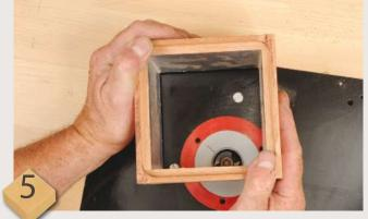
The top and bottom are rebated in. Set up the router table with a small rebater at about half the depth of the top. Place the box over the static cutter, switch on and push the box against the cutter in the direction of cut, working all round, then do the same on the bottom. Then fit a larger rebater and repeat for the top and bottom – two cuts make the operation much easier
