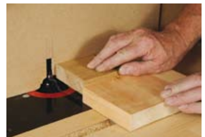
Using a supporting piece to help cut small components on the router table
