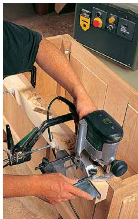
Routing hinge sockets – note bar clamped to chest to provide router with a running surface
