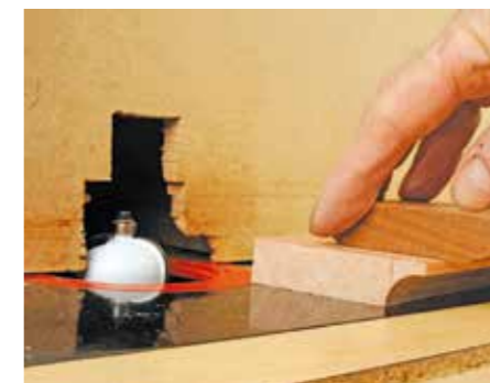
Making a cornice building up stage by stage, here checking the first two stages look right together
