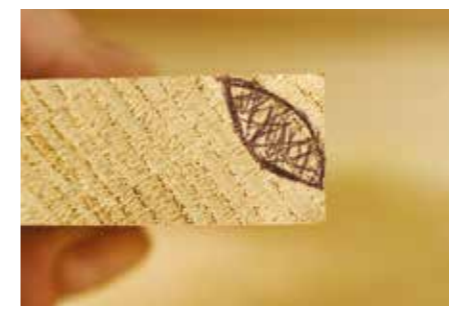
This rough drawn-in end illustrates how a roundover cutter removes less wood than a cove cutter. The latter will need more passes, taking off less wood each time, to avoid straining cutter and machine
