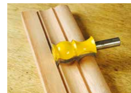
A tall face mould suitable for corning using just the one cutter or for a moulded surround. Cutters like these are only available with a 1/2in shank
