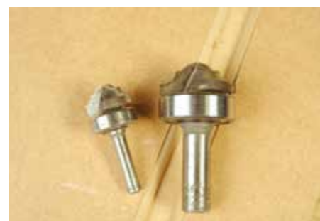
Face mould cutters which need to run around a template for a properly guided and accurate result. Dust is an issue especially with MDF, so extraction has to be fitted to the router
