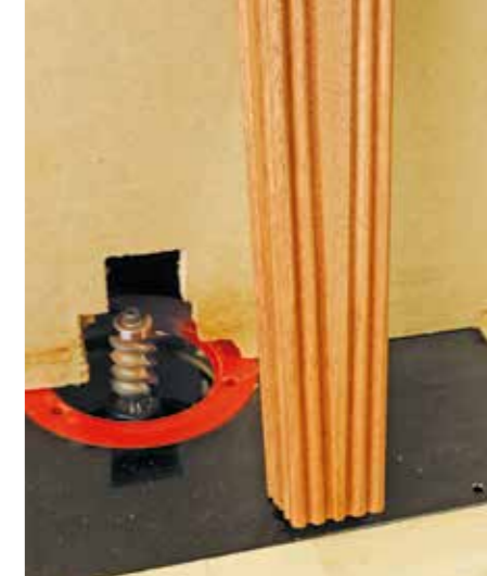
A tapered leg moulded using a multi-reed cutter. The trick is to ensure a neat corner meeting of the reeding on all four faces
