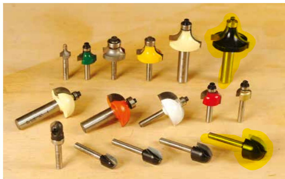
These very common profiles illustrate size variations very well, with larger ones on 1/2in shanks for strength
