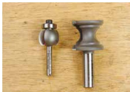
Two cutters, the left hand one being more suitable for a modern, gentle face mould and the right hand cutter designed for a traditional mould on the front edges of shelves etc., but needing guidance
