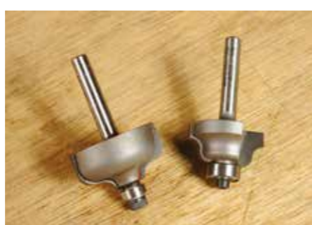
Two slightly different ogee cutters, generally associated with classical forms so better with traditional furniture styles
