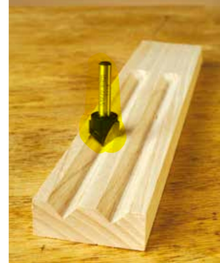
A V-groove effect works well here in ash. It could also be done with a round bottom corebox bit instead
