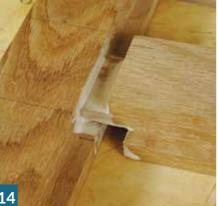
L5 The whole frame was glued and clamped together with the lower strap dry fitted and clamped in place. Then the frame was measured corner to corner to check it was square and then the frame was left on a level surface to dry so it would stay flat.
