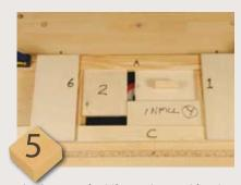
The first vertical line to be machined needs the numbered and lettered blocks shown here. The door blank has a grip handle glued to it to allow for drop-on cuts. This set-up makes the outer side of the topmost right-hand panel. Note the infill marked 'Y' which prevents sideways movement. To make the same outer line for the panels below, two more blocks and the infill are needed
