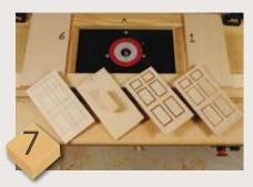
The key to making all the blocks for this jig is to work through the process logically, working out each step of the sequence. The result is quite satisfying, starting with a prototype door, then some identical size blanks with a handle glued on the reverse, machining the door, and finally sanding ready to paint. When completed, I find the result is really quite impressive
