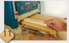
Thicknessing stock down thin enough for mouldings can be helped by fitting a false bed so you can go below the thicknesser's minimum capacity
