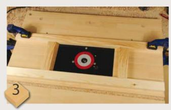
Fit a small straight cutter, say 2.5mm, in the router and lay the prototype door on the cutter so it is centred on the outermost vertical door line. Now clamp a batten running alongside the door. Move the door towards you so the cutter centres on the opposite outermost vertical line, and clamp that batten exactly parallel to the first one – this determines the width of the jig. Repeat the process for the length, cutting two battens to fit between the ones you have clamped
