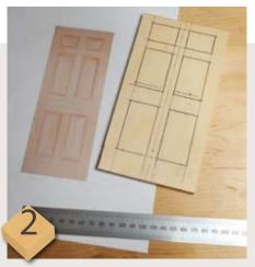
Start by designing the door using reference material to suggest proportions. The standard dolls' house scale is 1/12th so that is what we have used. When you are satisfied with it, run your marking out right across and on the edges too – this will help when setting out and building the jig
