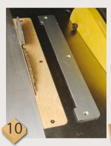
You may need to replace the insert plate on your tablesaw with one that fits tightly around the blade and riving knife, otherwise the tiny mouldings will just get dragged down the gaps
