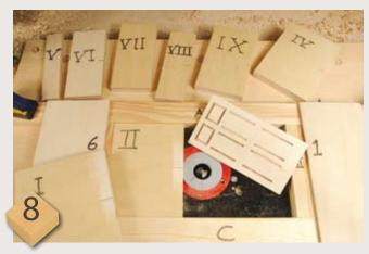
Using the series of crosswise blocks, machine all the slots using the drop-on technique for all of them. Working carefully, I managed to make a series of doors, each one taking under 10 minutes - if I got into the rhythm I'm sure it would be less. Once you master the thinking behind the process, it becomes fun and you can turn out doors until the cows come home, it's a job done
