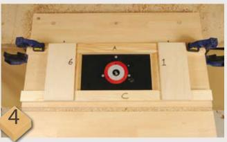
Ensure the jig is exactly square and glue and pin two pieces of thin ply on the outside ends of the jig – this will lock it rigid ready for the rest of the process. The numbers and letters relate to the door machining sequence. The machining problem we need to address is that we have to create six frames, in three sizes, in two vertical lines down the door. We need absolute control or the door blank will wander about and the result will be a mess
