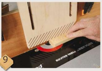
When machining small mouldings for the dolls' house, do it on the edge of a wider board and use sprung fingers and a breakthrough fence to give good, safe support. Then cut the moulding off on the circular saw and repeat the process to make more mouldings
