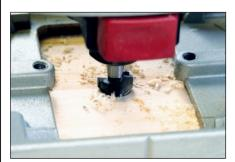
The cutter bodies have a black Teflon coating to reduce resin and chip build-up
