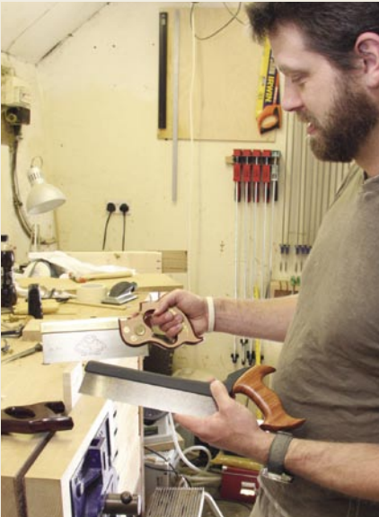
Contemporary The new Veritas Dovetail Saw (above) is a remarkable innovative shape that is really comfortable in the hand. It feels very balanced. Steve says it feels quite like his Lie-Nielsen model. He also tried an English Pax saw, and found them all to be perfectly good. But he feels the English saws are a little more clunky, and was attracted by the ergonomics of the Veritas. It certainly feels fabulous in the hand and cuts well
