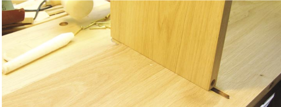
Joints In the end we decided to screw and glue the display unit to the top of the base unit (above being drilled for fixing holes). The plate racks are dovetailed into the central dividers (left) with little grooves on the other side for the glass shelves. The central dividers are housed in the top (below) with stopped housings
