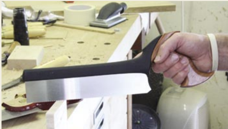
Contemporary The new Veritas Dovetail Saw (above) is a remarkable innovative shape that is really comfortable in the hand. It feels very balanced. Steve says it feels quite like his Lie-Nielsen model. He also tried an English Pax saw, and found them all to be perfectly good. But he feels the English saws are a little more clunky, and was attracted by the ergonomics of the Veritas. It certainly feels fabulous in the hand and cuts well
