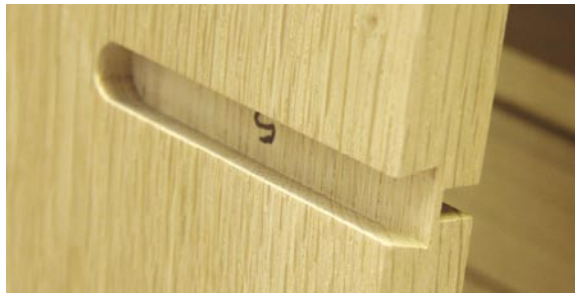
Joints In the end we decided to screw and glue the display unit to the top of the base unit (above being drilled for fixing holes). The plate racks are dovetailed into the central dividers (left) with little grooves on the other side for the glass shelves. The central dividers are housed in the top (below) with stopped housings
