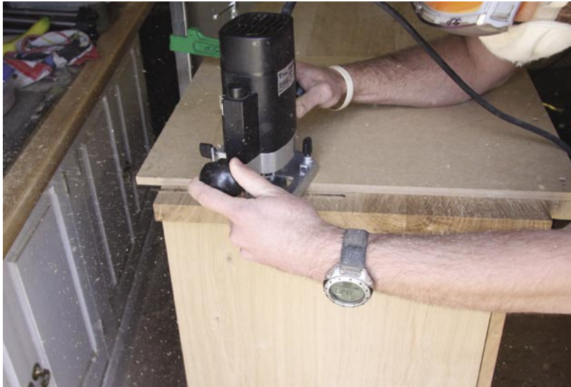
Transport The top of the base unit being grooved for the display unit. Steve uses a guide bush with wide T-square to give a good platform for the router
