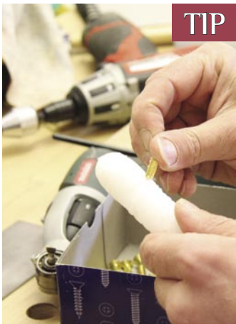
Waxing Brass screws will enter oak easier if you wax them first
