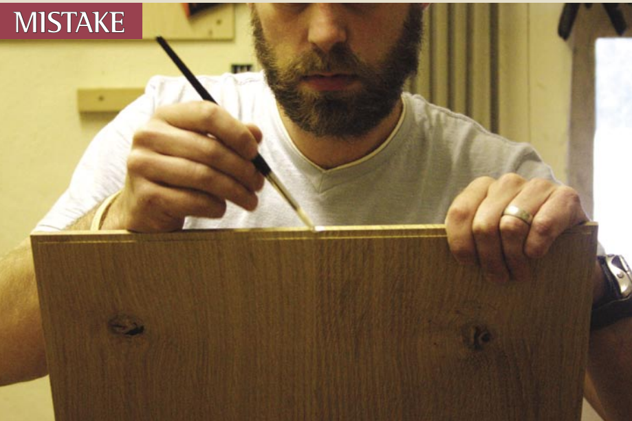
Assembly To allow the panel to move in the door you only glue at the centre of the panel (above) on the endgrain. That way the panel can expand and contract into the grooves, but doesn't rattle. Steve made the schoolboy error of putting glue on the panel, which then gets smeared out onto the panel, rather than on the rail, where the glue gets forced into the groove
