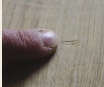
Bruise Somehow in the tight confines of the workshop the top of the base unit got bruised. If you plane this back without trying to coax the depression up, the bruised fibres may rise again later
