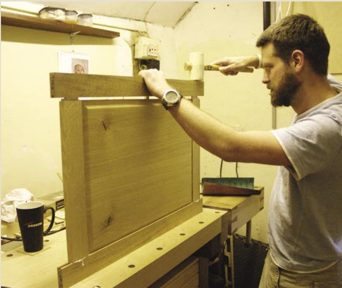
Alignment Although Steve will use a rubber mallet to knock a stile onto the tenons, the panel needs to line up perfectly so that it's a push fit into the groove around the inside edge of the door parts
