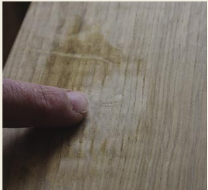
Solution The iron will pull up most of the bruised fibres, and then it's just a case of scraping back a little
