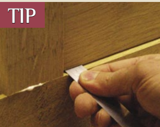
Tweaking Steve uses a metal rule to move the door panel a fraction to get it exactly in the right position. "There's many a use for a 6in rule beyond measuring," he says from time to time
