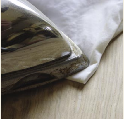
Ironed By using a damp cloth and an iron you can coerce the bruised fibres back up again, but take care not to burn the wood
