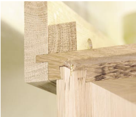
Cornice The cornice is fixed to the top with a tongue (below) on the top of the display unit and screw blocks. The back boards fit into a rebate around the back of the display unit
