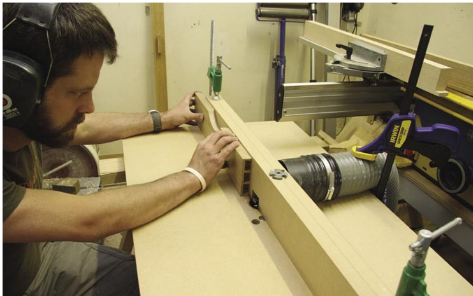
Harmony Steve's drawers are a harmonious combination of hand and power woodworking. He uses a Woodjoy Precision Dovetail Template (top, £14.63 from Classic Hand Tools) to mark out the tails and a Wealden (wealdentool.com, 0800 328 4183) slotting cutter to machine the groove in the drawer front for the drawer bottom
