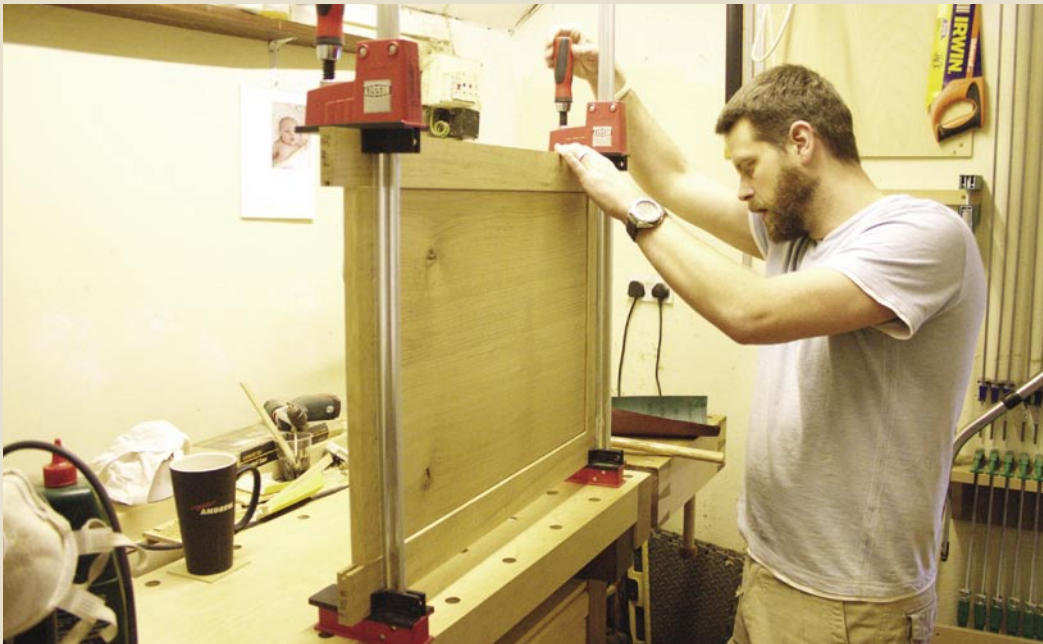
Tweaking Steve uses a metal rule to move the door panel a fraction to get it exactly in the right position. "There's many a use for a 6in rule beyond measuring," he says from time to time
