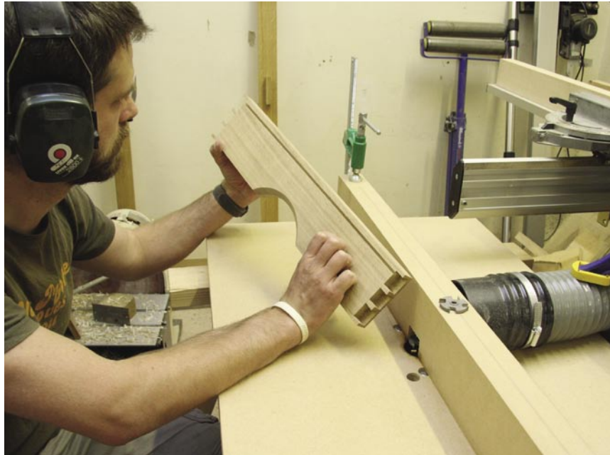
Harmony Steve's drawers are a harmonious combination of hand and power woodworking. He uses a Woodjoy Precision Dovetail Template (top, £14.63 from Classic Hand Tools) to mark out the tails and a Wealden (wealdentool.com, 0800 328 4183) slotting cutter to machine the groove in the drawer front for the drawer bottom
