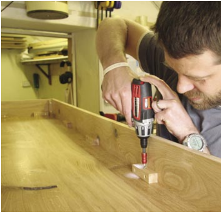
Cornice The cornice is fixed to the top with a tongue (below) on the top of the display unit and screw blocks. The back boards fit into a rebate around the back of the display unit
