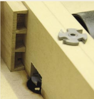
Wealden Steve used a Wealden slotting cutter on an arbor to slot the drawer front
