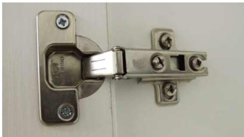
Concealed or kitchen hinges are used in mass production and knock down furniture as seen in this kitchen cabinet
