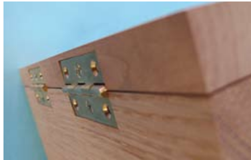
The door opens to 180° and is flush with the inside of the cabinet
