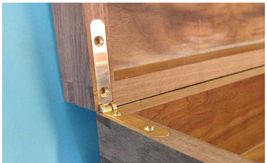
The hinge is ready for screwing in and the box needs sanding and finishing
