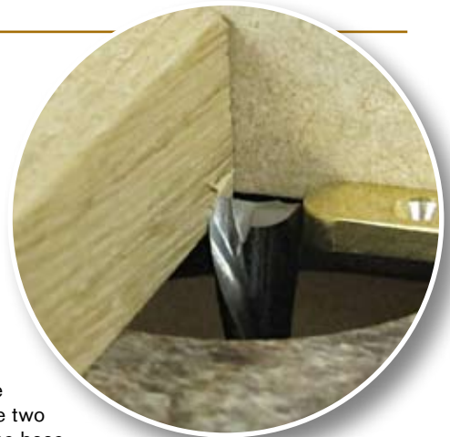
Setting the cutter height to the leaf thickness
