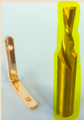
I use a spiral down-cut router cutter to fit my SmartHinges
