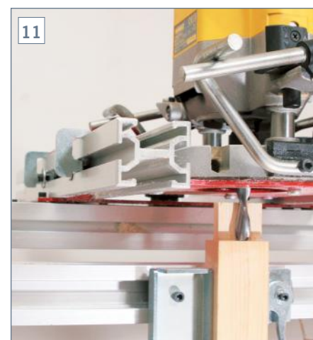
Cutting a tenon. Note spiral cutter
