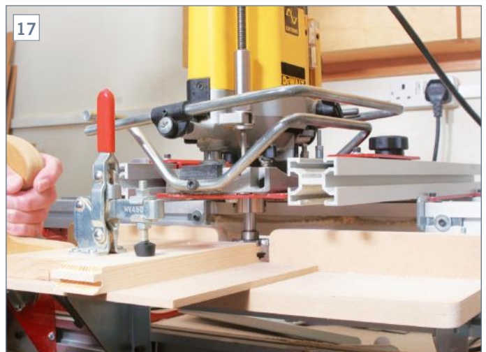
Scribing a door rail. Note home-made carriage
