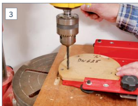
Drilling the router plate to take the DW 625
