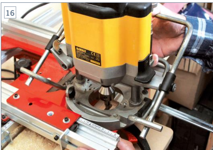
Mortising. Workpiece clamped to table fence. Note use of the PlungeBar
