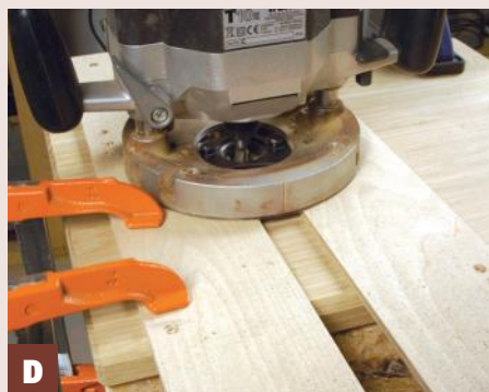
D The clamps need to be moved one at a time so as not to move the jig out of place
