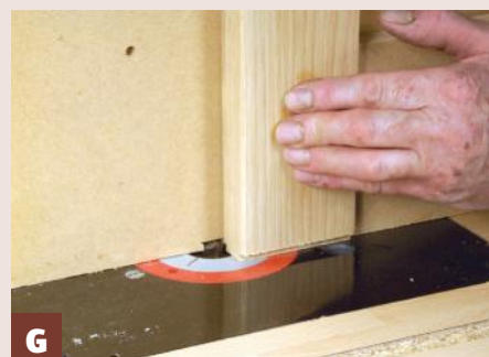
G The stretcher is being pushed by an MDF block behind to keep it upright
