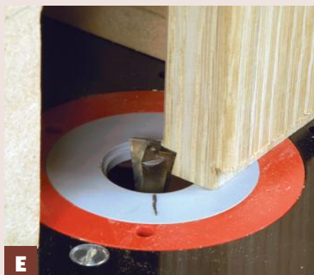
E The cut needs to be adjusted carefully from both faces
