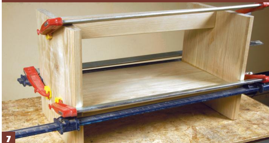
7 Long-reach cramps are needed to hold all the components tightly
