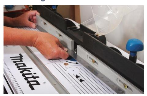
▲ A bearing on the Trend biscuit cutter being lined up with the table fence
