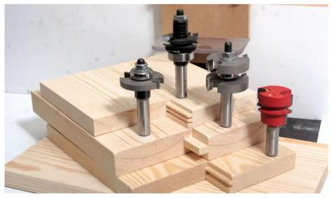
Three special joint cutters and joints made with them
