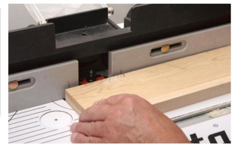
Pivoting the board into the cutter. Note pencil marks on fence. The guard is raised here for photographic clarity
