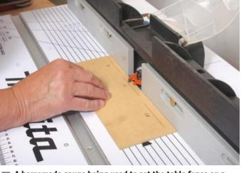
A homemade gauge being used to set the table fence on a non-bearing slotter
