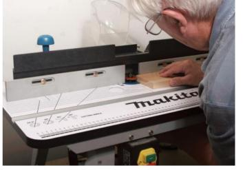
The cutter being set to the middle of the board
