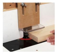
Cutting the groove with the cut centred in the board thickness
