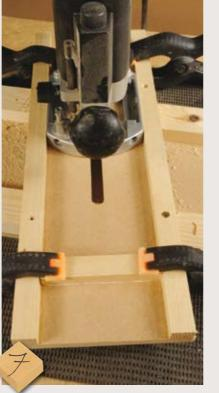
Glue end stops to limit the router's travel each time. Your jig is complete, apart from the registration stick slots which will be formed later
