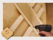
Screw the router tray on one of the angled lines. The tray must be long enough for the router to move right across the lower tray
