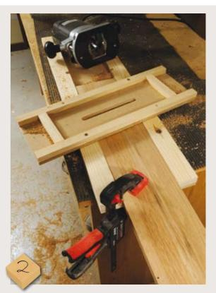
Continue until three slots are done, so the first slot appears from underneath the router tray
