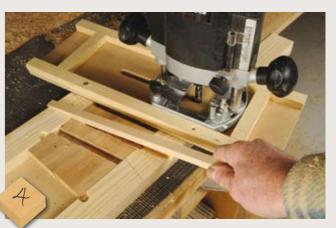
Refit the router tray and replace the test piece. Make up a registration stick that fits tightly in the batten slots and second CD slot. Now make the next and all subsequent slots using only the registration stick
