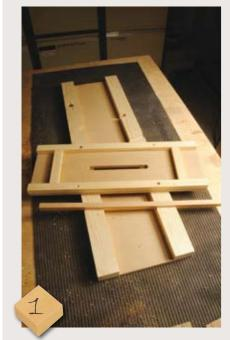
The jig consists of two trays – one for the components to slide in and one for the router to slide in. The latter is screwed to the component tray and a registration stick ensures all the slots are the same distance apart
