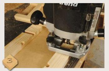
With the test piece still in position, mark across the side battens where the first slot is. Remove the router tray and use it as a temporary fence for the router. Remove the test piece and rout slots through the side battens
