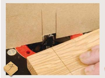
Set up a large diameter straight cutter to machine the back panel rebates. Aim to set the panel in by about 0.5mm it is better that the solid sides protrude fractionally.
