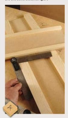
Mark across halfway along the component tray, then set an adjustable bevel to about 78° - which looked about right. Mark this angle on both the left and right of the centreline as the jig is reversible
