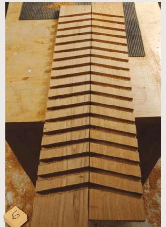
Now unscrew and move the router tray to the already marked opposing angle and repeat steps 1-5 - excluding the use of a test piece, as you will have demonstrated to yourself that the method works. You should end up with two mirror matched sets of slots waiting to be trimmed to length
