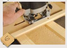
Fit a 12.7mm straight cutter in your router, sit it in the upper tray and do a plunged slot cut through the router tray base so it starts and stops halfway into the side battens
