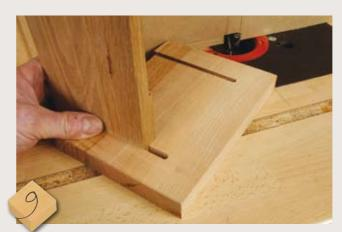
You can only do the right-hand slots like this, the other two need to be done running from the outfeed side. Don't worry, you will not be climb-cutting - we aren't widening a slot, so which ever direction we approach the cutter from doesn't matter. I machined these slots with the stop block to the right and found it safe. Refit the large straight cutter and rebate the ends of the sides to form the tongues. Trim off the leading edge of each tongue so it fits in the stopped groove
