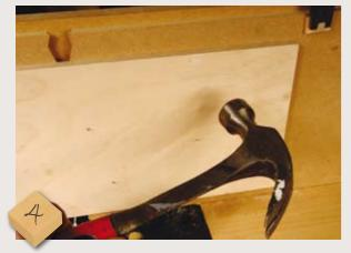
Pin the board to the sub fence ensuring each component can slide underneath without riding up as it passes over the cutter
