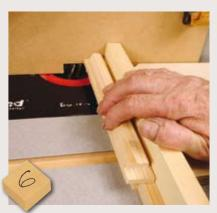
Assuming all components are successfully machined, the stub tenons need to be formed on the glazing bars and top and bottom rail. Fit the rebate cutter and set the height and depth with a plain sub fence in place. Use the push block to support each component, but this time use a slim, loose fillet of wood to fill out the rebate nearest the pushblock so it gives proper support
