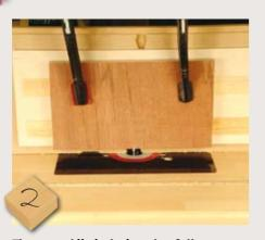
The second jig is designed to fully support each glazing bar after the rebates have been machined on the reverse side. This operation removes a lot of wood so there has to be a way to preventing vibration, tearout and a component turning over as it feeds through – all while keeping the operator's fingers safe
