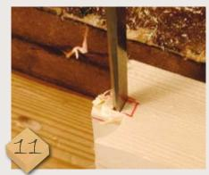
The rail tenons have their outer corner chopped away to fit the haunched mortise. Check the fit of all tenons before glue-up and final assembly
