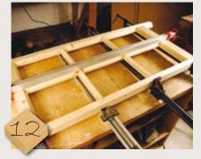
Clamp the window frame up tightly and check for square and that it isn't twisted. Clean up the glue, unless you use PU glue as I did, in which case clean up only once it has set hard
