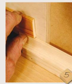
Now, find some slips of wood that are the same thickness as the wood between each rebate. Providing all components are machined to the same thickness. they should all be able to slide through without getting stuck
