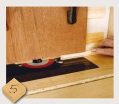
Now, using the second jig, the moulding profile is machined. The cutter needs to be set at the correct height to match the already scribed ends. The sub fence, complete with attachments, is clamped in place and the glazing bars are run underneath, first checking with a test piece that the cut width is correct. Note the stiles and rails are machined without the front board on the fence
