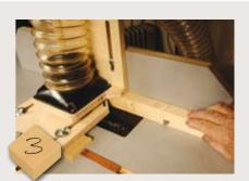
This apparently complicated rebating set-up consists of a large bore extraction port, also acting as a hold down, and spring fingers for sideways pressure, clamped firmly so it cannot slip (see WPP50 Mini Projects). Note the spring fingers are raised up on 9mm MDF, so pressure is applied at mid-height of the glazing bars as they are rebated. One short glazing bar is used to propel the first one through and so on, thus making for safe, controlled machining
