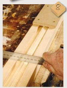
Lay out the components and measure and mark where the mortises need to be. Bear in mind that the rails will fit into haunched mortises, i.e. they stop short of the ends so the rails are locked in place and cannot simply slip out of place. Fit jig number three over a stile, press the top board down, and check the open end is flush with the top while clamped in the vice
