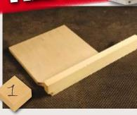
Because of the complexity of making window frames, more than one jig is required. First up is a perfectly square pushblock as described in WPP50 Mini Projects. This simple device is an underrated, but very effective, aid. It safely supports each component being scribe cut without any need for the table fence to be parallel with the table itself, as would be the case with the mitre fence
