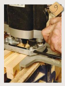
Machine the mortise to depth using just one fence and, in this case, a 6.4mm straight cutter. The mortise ends are chopped square with a narrow chisel
