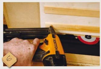
Pin the lower strip so each component can just slide under without any play. The upper strip is there to hold the front board, which is added last. This will trap each glazing bar, preventing any sideways movement and avoiding any supporting finger contact. The front board is added last
