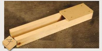
The third jig is very simple. The purpose of it is to fit tightly around each frame component, including the glazing bars. The top board is the height register so the two battens should always sit level with the moulded edge of each glazing section. This creates a sort of mini mortise box that the router can sit on, to machine the stub mortise holes. The open end allows working at the ends of the frame stiles and is clamped tight to prevent slippage
