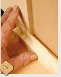
So, to start, machine the rebates on your test piece and find or plane a board to the same thickness as the rebate width. Check the test piece sits squarely when the board is positioned on the sub fence
