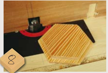
The finished bottom with a tongue formed all round. Check it fits the side grooves before assembly
