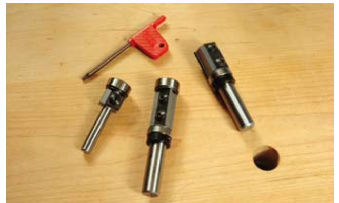
Instead of resharpening cutters, it's possible to buy replacement tip blades
