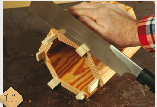
The loose tongues are trimmed off flush and the planter sanded to a finish all round ready for a varnish coat
