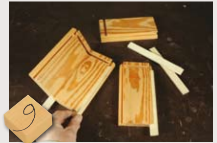
The loose tongue position which stops short of fouling the planter bottom when inserted
