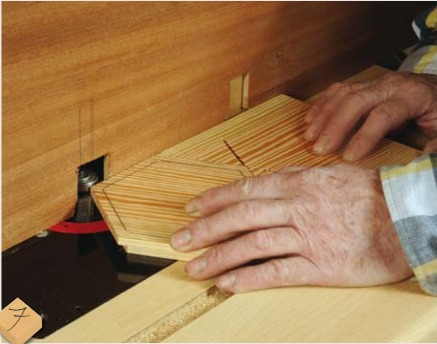
The bottom has its tongue formed using a rebate cutter and a breakthrough fence for safe, even working. Note the waste from cutting out the bottom is used as a perfect push piece
