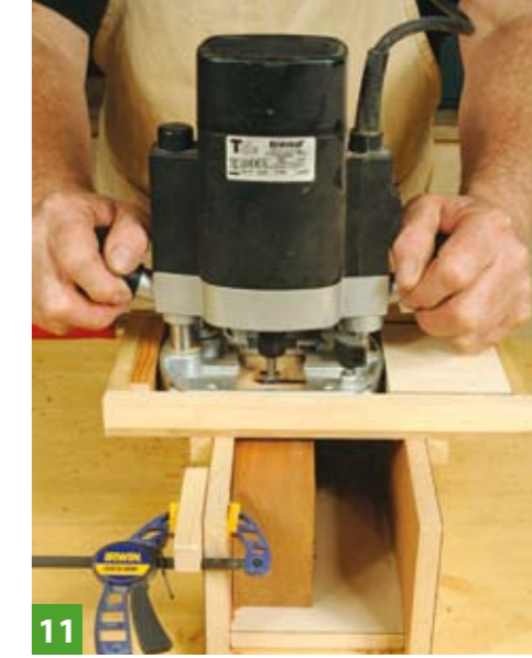
11 Most of us don't have a chisel mortiser so a router and mortise box makes perfect sense. You can even mortise tapered and angled components
