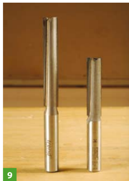
9 The right-hand straight cutter is a typical length but for safety is much shorter than the 'honeycomb' cutter on the left
