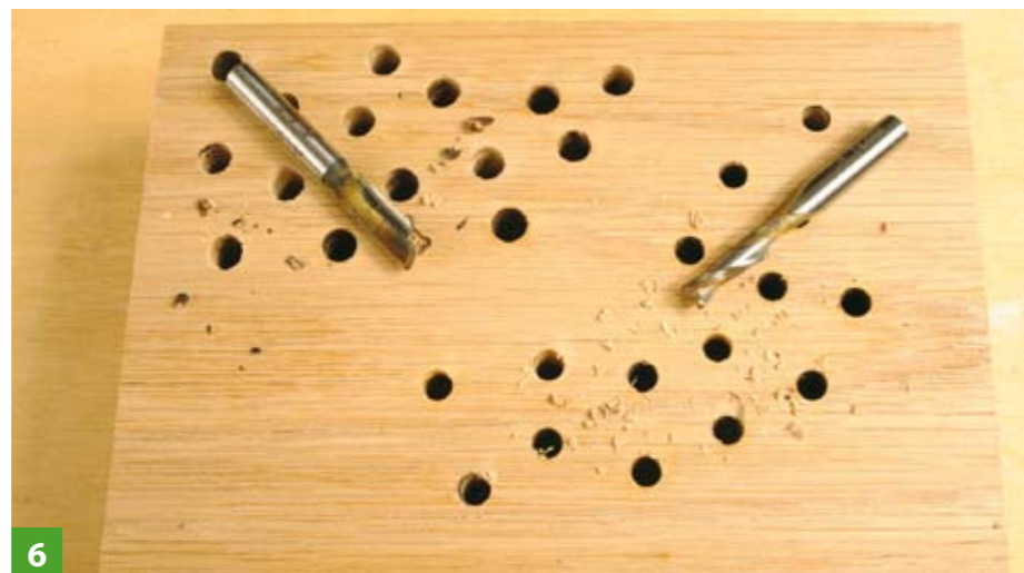
6 The left straight cutter has created a lot of burning and heating of the cutter creating stuck on deposits. The up-spiral cutter is left in a much better state after machining its holes
