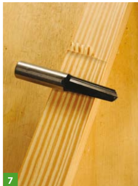
7 This taper cutter creates a very subtle slope which could prove useful for more than just mould making
