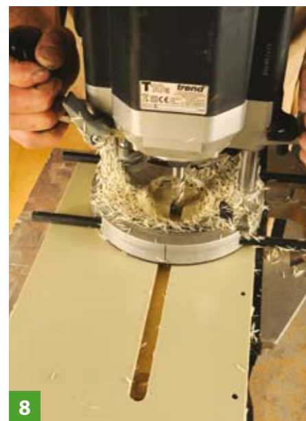
8 Cutting plastic materials can create excess wear and uneven edges whereas a specially designed cutter will be much more suited to the work
