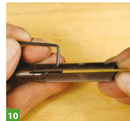
10 If you do a lot of repetitious machining of hardwoods and manufactured boards, a replaceable tip blade makes sense
