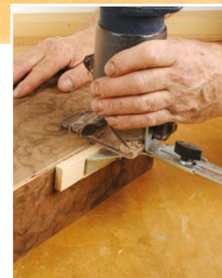
Machining to fit stringing using a trimmer and a straight fence
