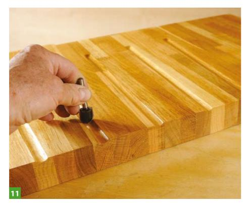
The corebox is ideal for creating sink water run offs on wooden draining surfaces
