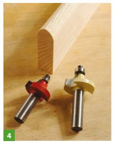
This is exaggerated but demonstrates the need to choose a smaller roundover and avoid a peak which ruins the job and means the finished profile isn't supported by the outfeed fence either
