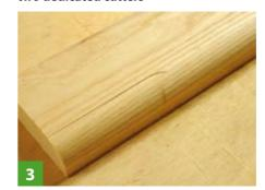
Always set the cutter depth up a fraction to avoid creating a ridge line that cannot be sanded out
