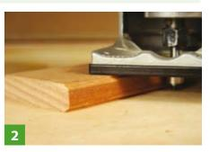
Even a roundover cutter can create a one step ovolo type effect as for a shelf shown here
