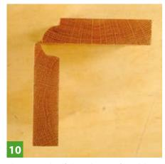
The principle of the rule joint for table flaps – flap hinges are fitted underneath
