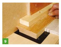
Cove cuts in particular need extra support to avoid the work chattering and the moulding being marred as a result of this
