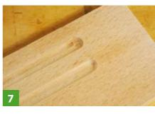
The top flute has a slight burn which is hard to sand out; it can often be worse than this, especially with a slightly blunt cutter - keep the router moving
