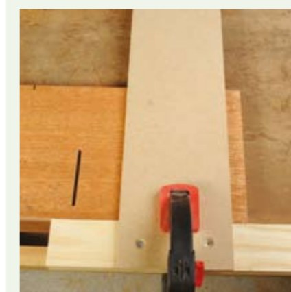
6 A 4mm straight cutter can create mid-panel slots
