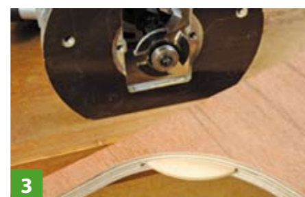
3 Working around tight curves
