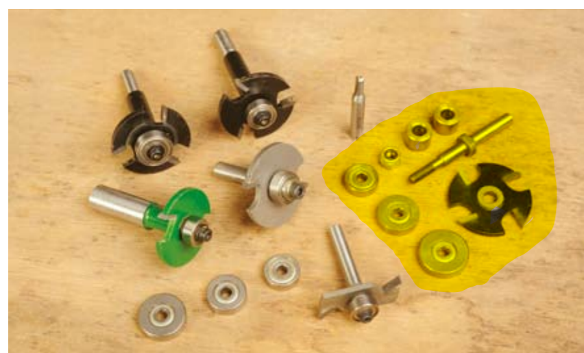
All 4mm groovers: (top left) Wealden biscuit cutters; (centre top) Makita straight bit; (centre left) Trend; (middle) Makita; (front) Whiteside; (middle right) Wealden with bearing and spacers
