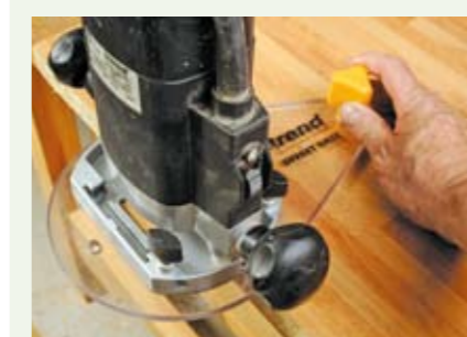
7 Slot cutters can be used to fit other more unusual biscuit components
