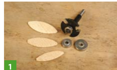
1 Capable of machining three standard biscuit slot sizes
