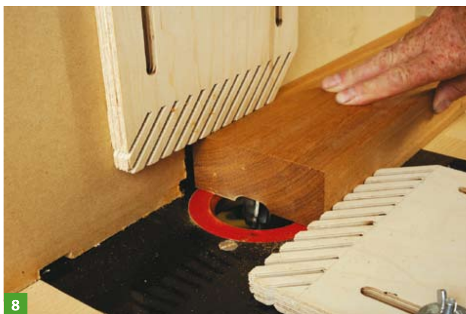
A facemould cutter can wander, so pressure fingers are needed
