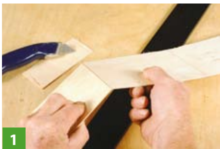
1 Score the laminate so it will ‘crack back’
