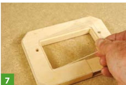
7 The polycarbonate is carefully trimmed to fit
