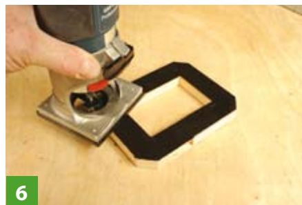
6 Trimming off the surplus laminate
