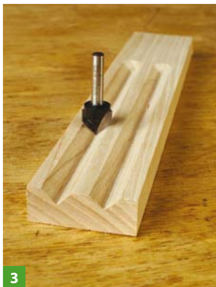
To obtain a 'stopped' effect, use a stop block clamped to the table fence
