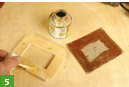
5 Apply contact adhesive to both surfaces
