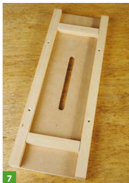
Tray jigs like this one control the movement of the router
