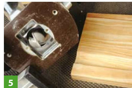
A straight fence can cause damage at the end of the workpiece
