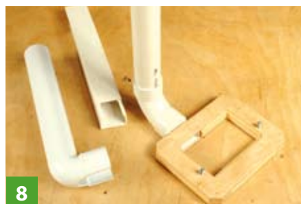
8 The white waste pipe makes the spout
