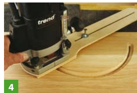
Use the last pass to clean away any burn marks present
