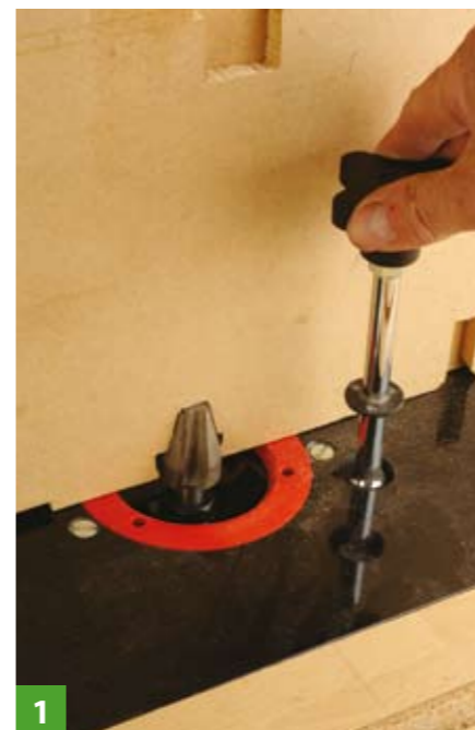
1 The through-fence on the router will prevent breakout
