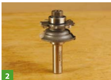
2 This cutter has to be reassembled when changing from profile to scribe
