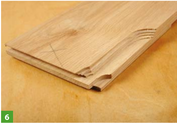
A test piece for panel raising
