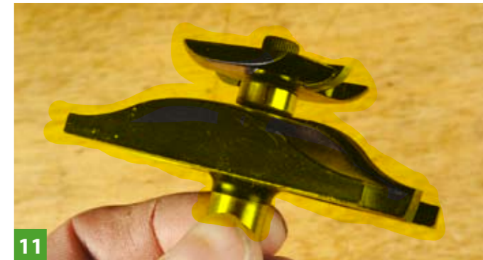
Right: The small back cutter creates a perfect tongue
