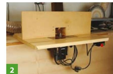
2 The WPP router table that I made works really well
