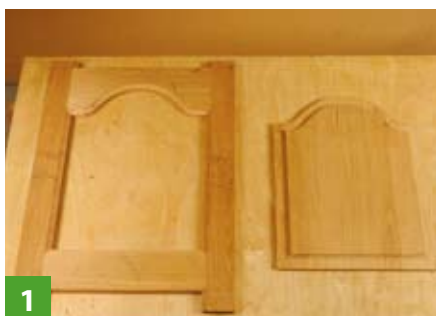
1 A typical frame and a matching panel for quick and easy construction
