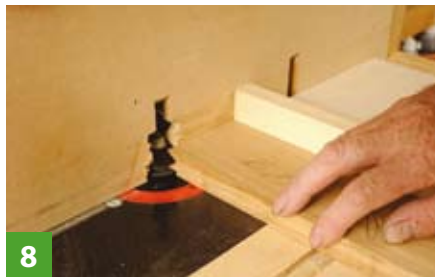
Scribing cuts need a through-fence for good support
