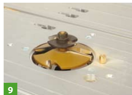
9 This panel raiser just fits in the table opening
