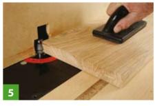
Edge moulding a board and then cutting each piece off means the new raw edge will need planing before the next moulding is done
