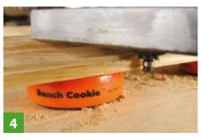
Bench Cookies are one of several handy non-slip work supports which allow cutters and bearings to hang down lower than the workpiece underside
