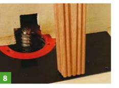
The result of moulding from both edges creates a visually pleasing effect especially when performed on all the adjoining component faces
