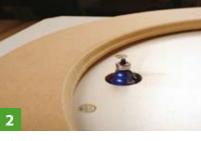
Take care in choosing the correct cutter size and minimising the required rebate depth, making sure you have enough running surface for the bearing
