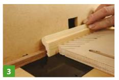
This guite ambitious bolection moulding - panel frame with rebate - needs plenty of support and multiple passes
