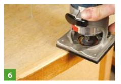
Any router is suitable, a small trimmer can be used one-handed for this work
