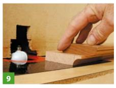
With just two stages machined you can get the idea that with further mouldings and alternating plain flat sections you can make an imposing cornice
