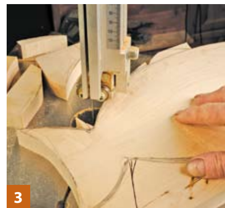
3 Allow the bandsaw blade to follow your line and not deviate. Also, do not force the wood
