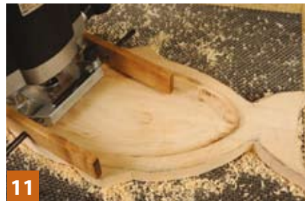
11 Lift the router off and with the power off push down hard and lock the plunge, then lower the router on the job and do a cleaning up pass
