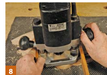
8 Holding the router firmly, make shallow passes starting near the outside of the dish shape
