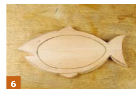
6 Next, mark the dish shape taking care to avoid the eye and the front of the head
