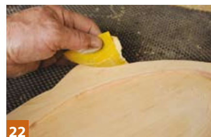
22 'Break' the edges with abrasive so the platter is safe and pleasant to the touch
