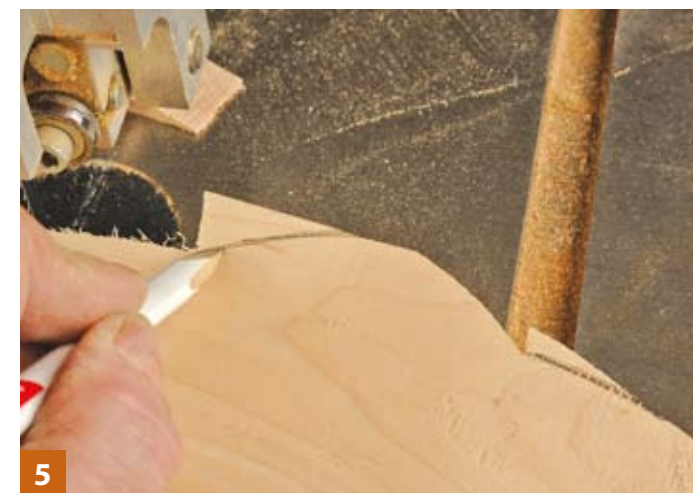
5 For cuts that can't be completed due to throat restriction, mark on the reverse of the workpiece and complete from that side
