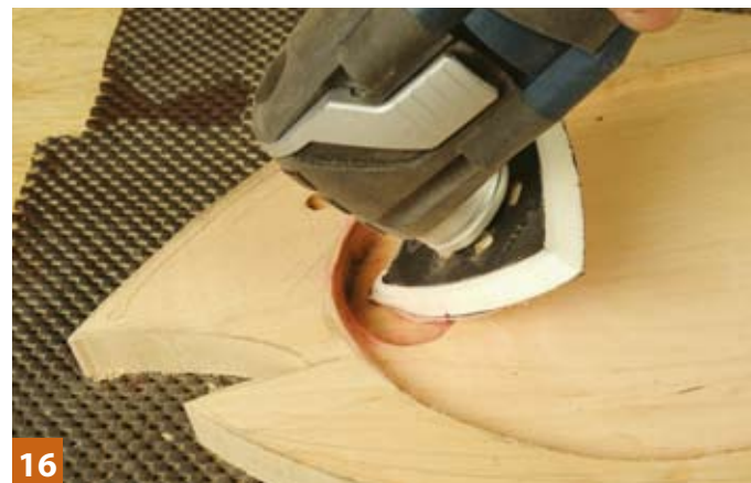
16 Use a delta sander and medium abrasive to sand the edges of the recess
