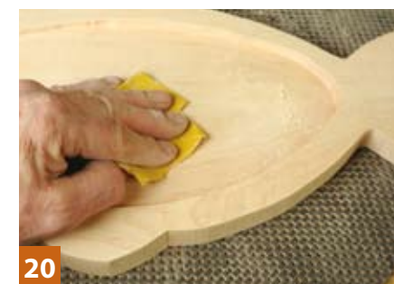
20 Give the platter a good hand sand to remove any final traces of burning
