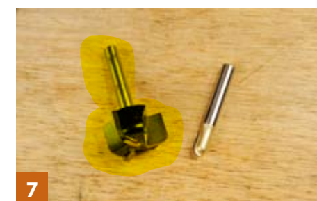
7 To shape the dish use a Wealden groundwork cutter with curved corners and a small Trend single blade corebox cutter for the eye
