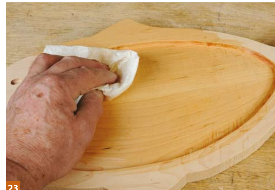
23 Finally, coat the platter with a wood safe finish or any food oil – the choice is yours
