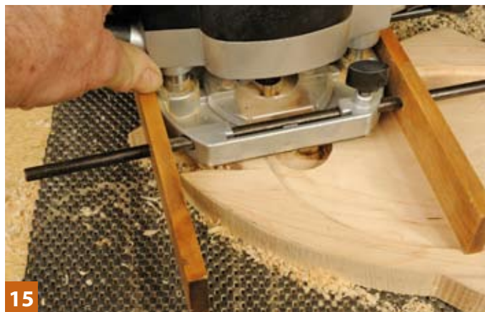
15 Use the small diameter corebox cutter for a shallow plunge to create the eye recess
