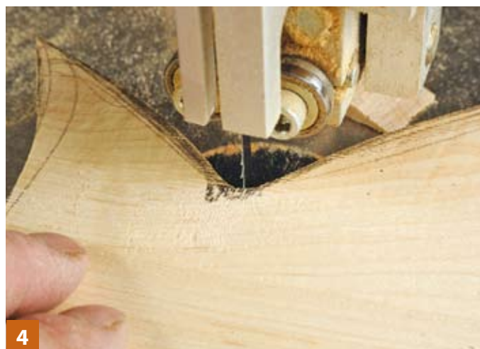
4 When working on tight inner curves, remove the bulk and use a sideways 'nibbling' action to tease away the remaining wood
