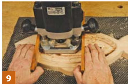
9 Remove the centre of the dish moving the router anti-clockwise into the cut direction
