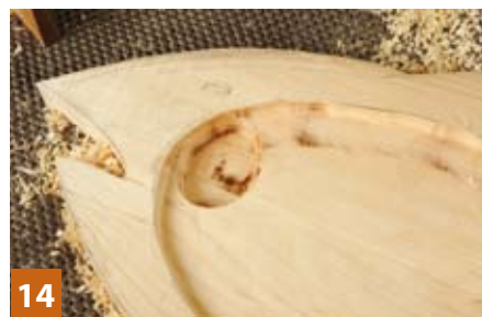
14 Remove any burn marks and ensure all food recesses and the eye have curved bottom edges
