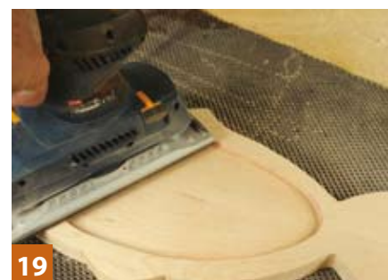
19 Use a standard orbital sander to smooth the rim and back of the platter
