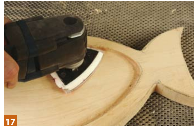
17 Again, use the delta sander for sanding the dished base including the radiused corners
