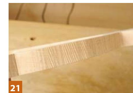
21 The bandsaw edges can be left as they both look and feel good to the touch
