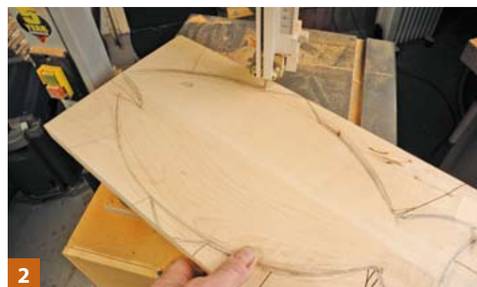
2 When bandsawing, allow plenty of relief slots so the blade doesn't get jammed during cutting
