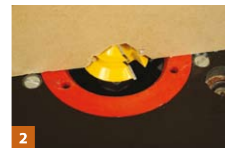
2 The lock mitre cutter gives a strong but very discreet joint
