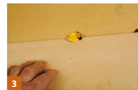
3 Sub-tables are often used with spindle moulders but they also work with router tables
