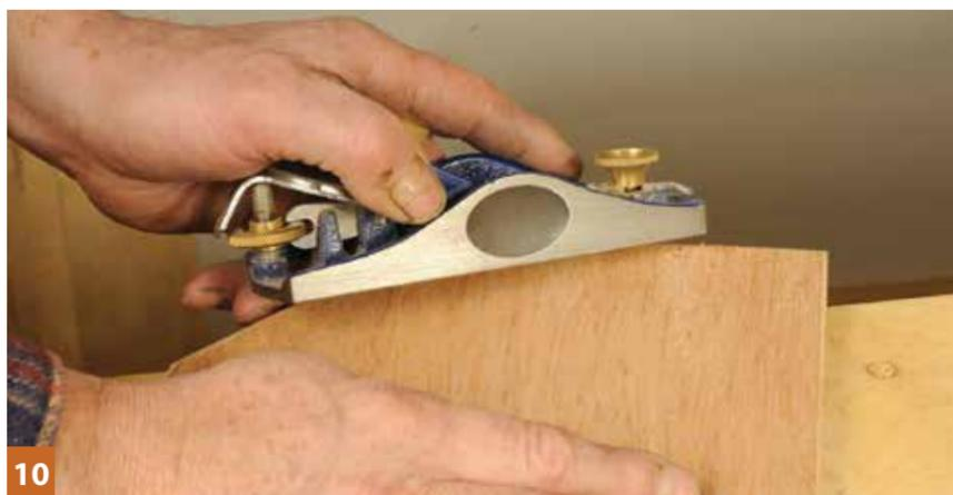
**10** In order to remove any grain tearing and get rid of sharp edges use a block plane to bevel the edges on both faces of the rack ends.
