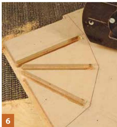
**7** The 12mm ply showing both lots of end slotting. The next job is to cut out the shapes.
