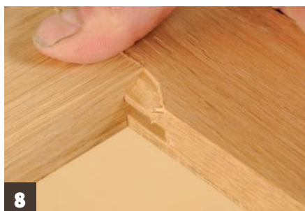
8 Do a test cut and check the faces are flush across the joint
