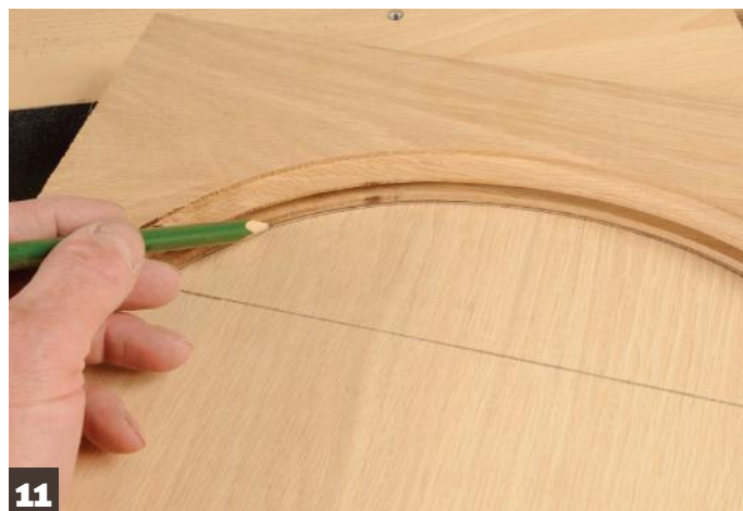
11 Marking out the arch shape on a panel blank. Next add an arc 9.5mm larger and increase the shoulder height by the same amount – this will be the tongue that fits in the frame groove
