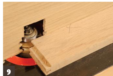
9 Place components with the 'seen' and to-be-moulded side downwards and mark the 'up' side on all components next to the edges that will be moulded to avoid machining mistakes
