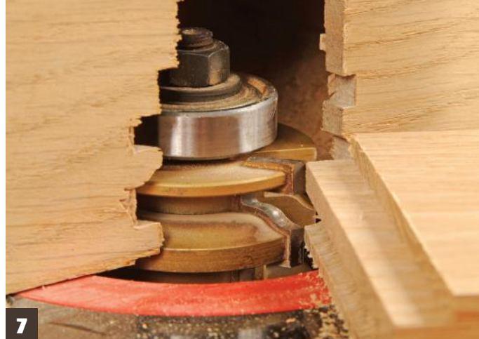
7 Start the process of profile moulding by lining up the mirror image part of the cutter with the already cut scribe part of the joint
