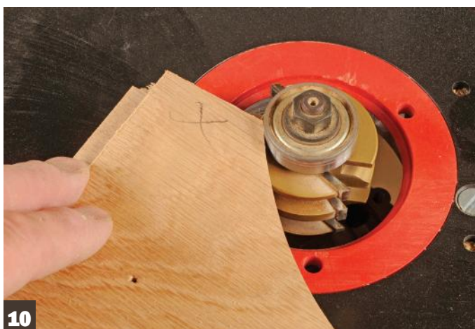
10 Machine the arch shape by bringing the left-hand tip of the arch (reverse face showing) into the cutter and moving it in a smooth motion across the cutter, keeping it pressed against the bearing
