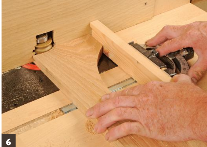
6 Doing the same operation on the already shaped arch top rail using the mitre subfence to support it properly
