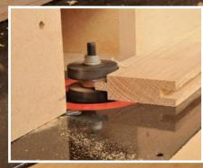
Machining a matching tongue profile – do test cuts to ensure a perfect alignment
