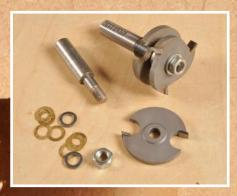
A two-part groover set for creating tongues and grooves in different widths. Showing the arbor, interchangeable groover adjustment shims, washers, and nut to hold everything in place safely
