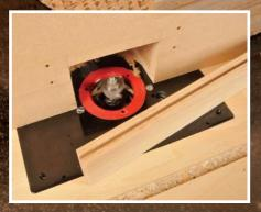
4 Slotting on the router table is easy, however, to avoid breakout as seen here, do a very shallow scoring pass first
