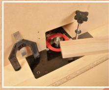
Accurate setting-up is required, especially if you want the groove exactly centred – a fine adjuster and a height setting gauge are needed
