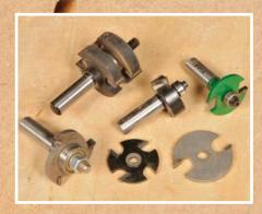
There are different size and types of groovers available, including the rebate cutter (centre) and the biscuit slotter (top right)
