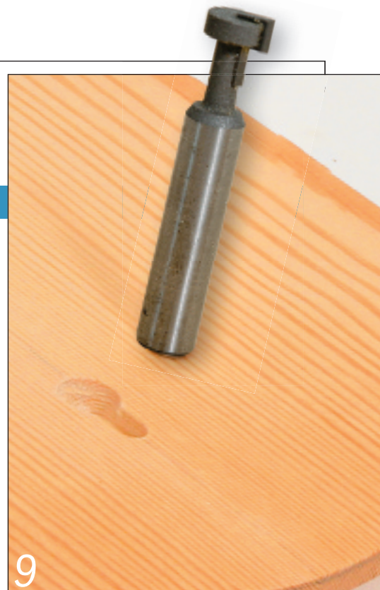
The keyhole cutter cuts holes for No 8, 10 or 12 roundhead screws
