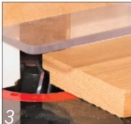
The smaller cutters can be used in the table or in a hand-held router
