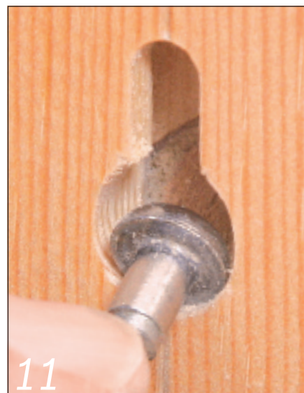
The keyhole fits over the head of the screw and drops down over it
