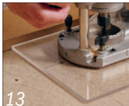
Use an auxiliary router base running against a straightedge
