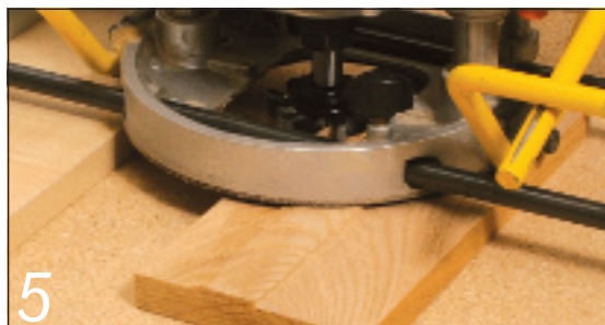
Run the router skis on a board at each side of the workpiece
