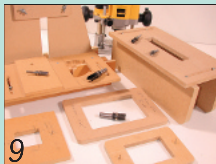
9 A selection of jigs and templates made with template profilers and straightedges
