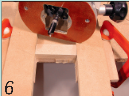
6 Clamp the workpiece and run the profiler around in a clockwise direction
