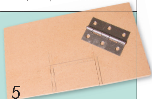
5 To make a hinge jig, draw the hinge and offset outlines on 9mm MDF
