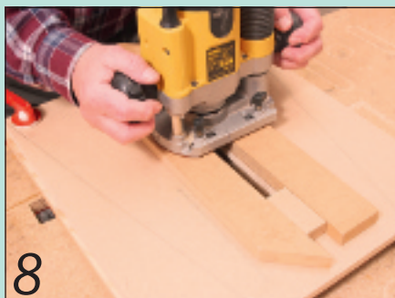
8 In this jig, the slot in the MDF had to be the exact width of the intended guide bush
