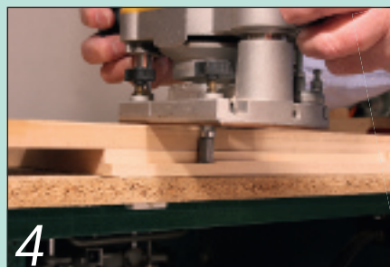
4 When rebating a panel, use a short profiler so you don't need a very thick straightedge
