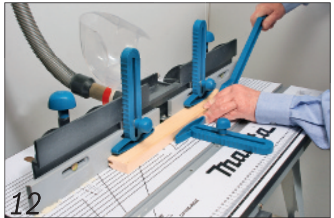
Profiling a stile; the vertical guard has been raised for clarity
