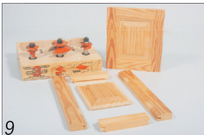
This CMT set can be used to make panels down to about 125mm (5in) square
