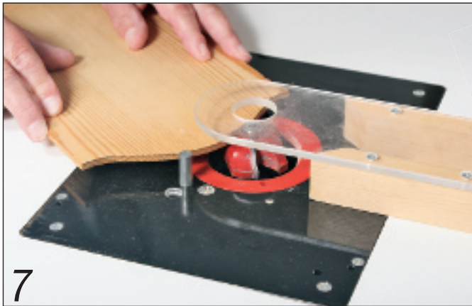
An arched panel being raised with a Titman horizontal panel raiser
