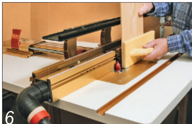
A panel being raised with a vertical cutter on an Inca table. Note the high 'wing' to keep the panel vertical
