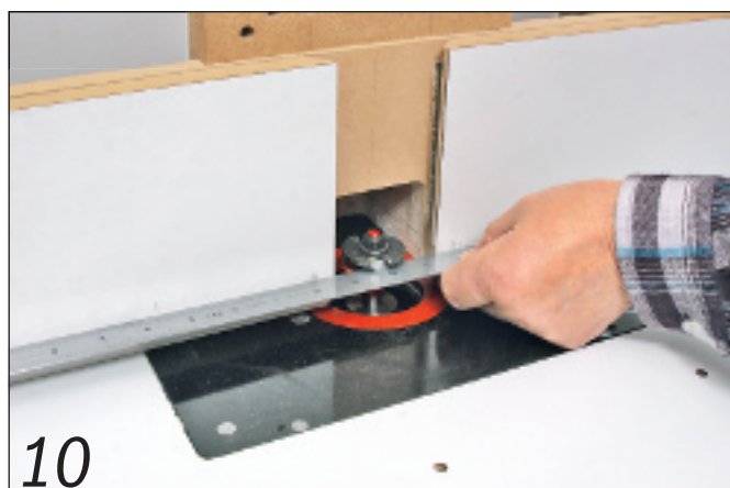
Lining up the table fence with the front of the cutter bearing
