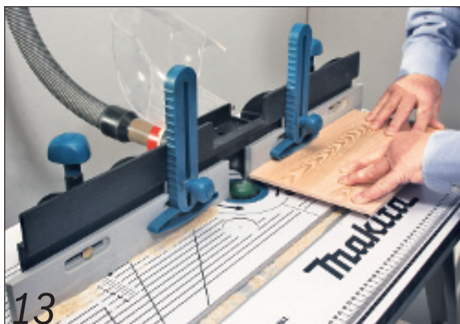
Raising the panel. Note the use of a non-bearing horizontal cutter
