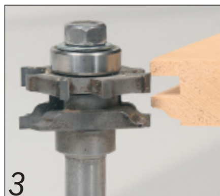
3 The same cutter configured for profiling rails and stiles
