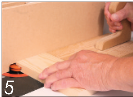
5 The drawer front is machined flat on the table with its inside face down...
