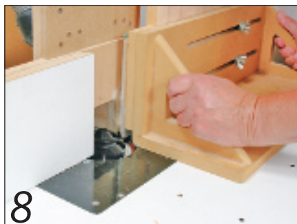
8 A vertical board is held in a jig for machining with the lock mitre cutter
