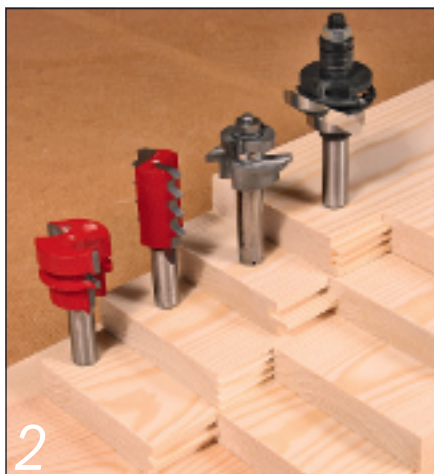
2 Four board joints, from left to right: CMT reverse glue joint, Freud raised panel V-jointer, Titman offset tongue-and-groove jointer and Wealden finger joint set
