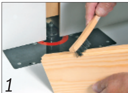
1 Removing feathering from the edges of a joint with a stiff bristle brush
