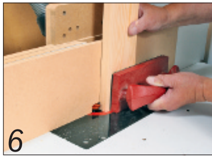
6 ...and the drawer side is machined in the vertical position with its inside face towards the fence
