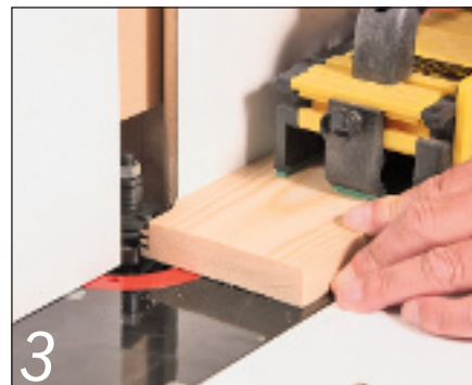
3 A 20 mm board being machined with the Wealden finger joint set
